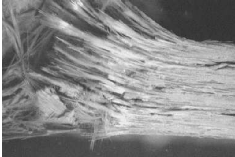
Figure 13 Damage zone in the not toughened material (B1)
