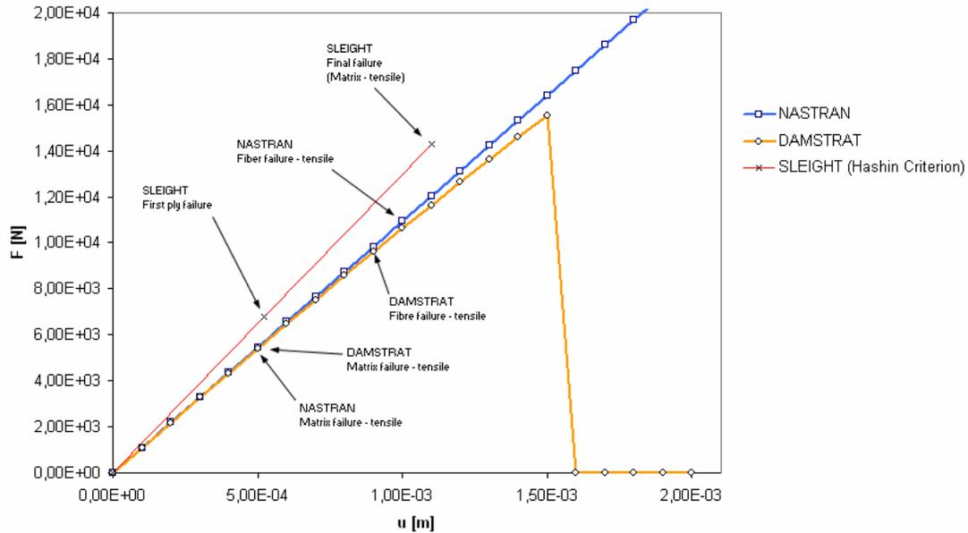
Figure 2: Tension load as a function of impose displacement for a tension-loaded laminate with hole.
