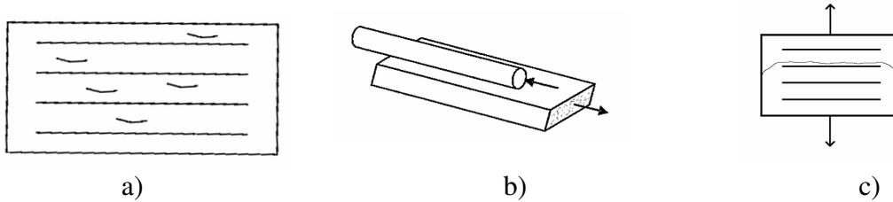
Figure 1 : Types of damage modelised by DAMSTRAT. a) Matrix microcracking. b) Fiber/Matrix shear decohesion. c) Brittle matrix tensile cracking. [4]
