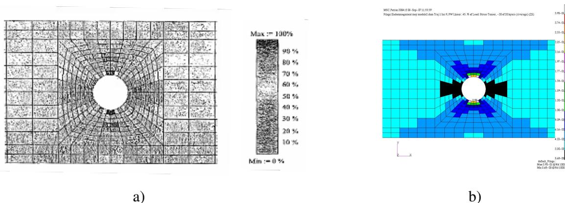
Figure 4: Damage at final failure for a tension-loaded laminate with hole. a) SLEIGHT [1]. b) d parameter - DAMSTRAT
