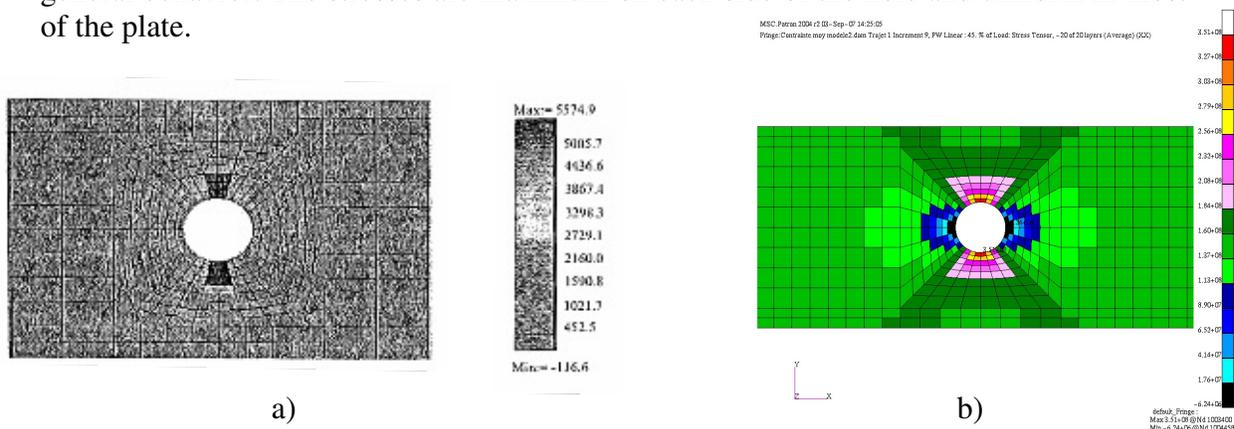
Figure 3: Tensile stresses at final failure for a tension-loaded laminate with hole. a) SLEIGHT [1]. b) DAMSTRAT
