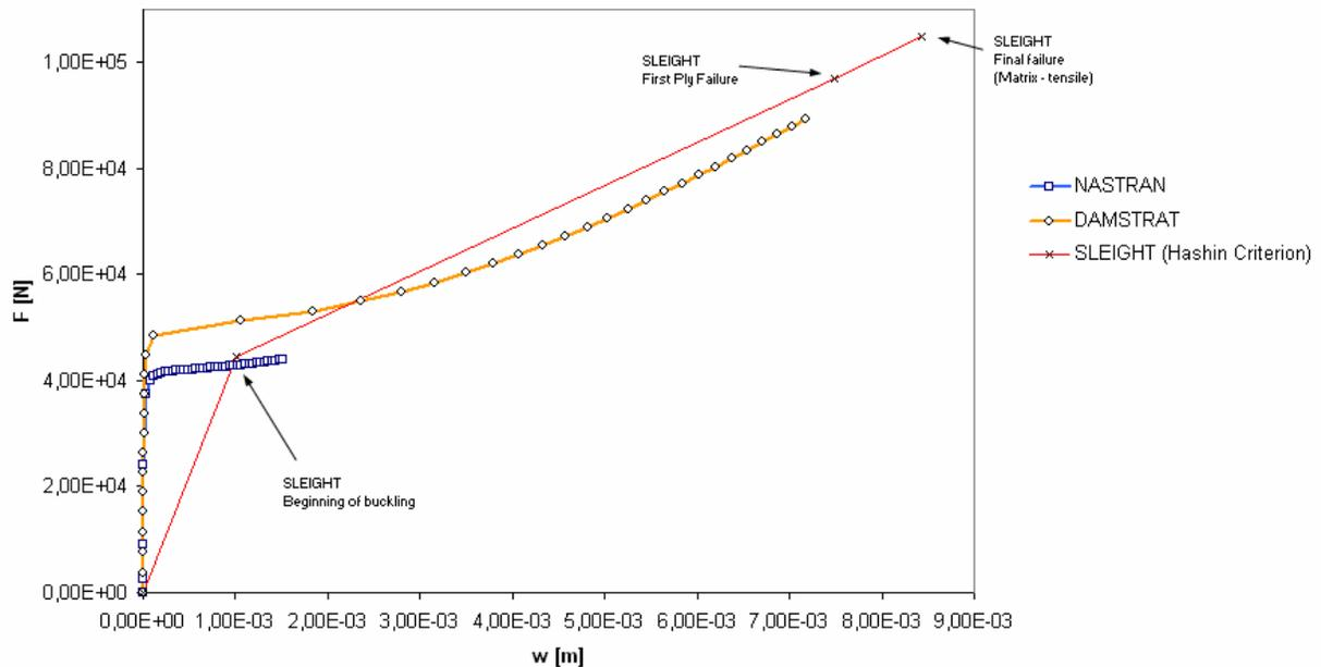
Figure 5: Out-of-plane deflection as a function of impose displacement for a compression-loaded composite panel.
