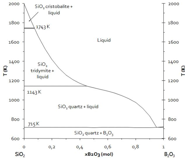
Figure 2 : Calculated  $B_2O_3$ - $SiO_2$  phases diagram
