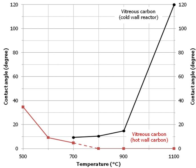
Figure 5: Variation of contact angle of  $B_2O_3$  on vitreous carbon as a function of temperature in Ar +  $O_2$  atmosphere.
