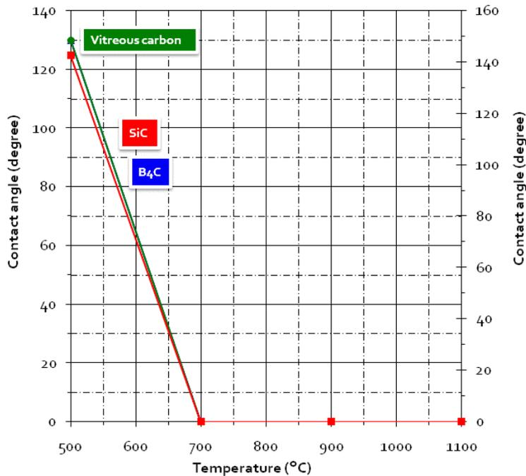
Figure 8: Variation of the contact angle as a function of T and nature of the substrate in Ar + H<sub>2</sub>O atmosphere.
