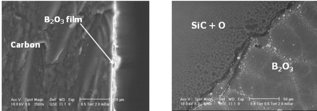
Figure 9: Morphological characterization of  $B_2O_3$  / carbon interface after thermal treatment at  $700^\circ C$  and top view of  $B_2O_3$  / SiC interface after thermal treatment at  $900^\circ C$ .
