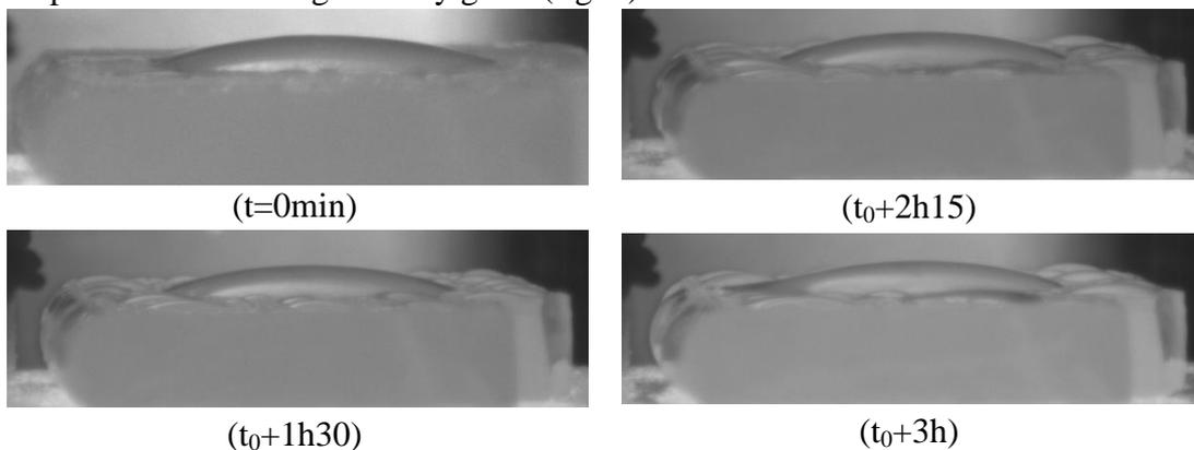
Figure 7: Behavior of  $\text{B}_2\text{O}_3 / \text{B}_4\text{C}$  system at  $900^{\circ}\text{C}$  in  $\text{Ar} + \text{O}_2$  in cold wall reactor.
