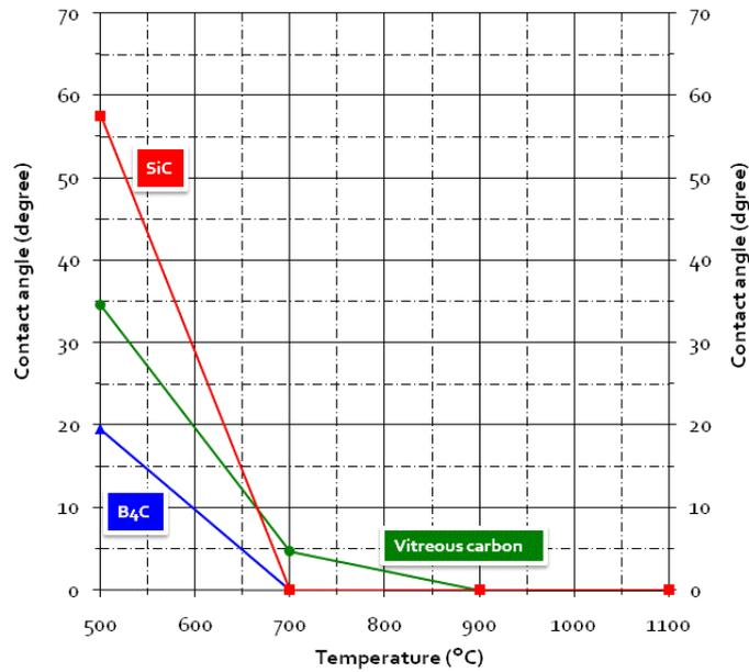
Figure 4: Variation of contact angle according to T and nature of the substrate under Ar + O<sub>2</sub> atmosphere in hot wall reactor.
