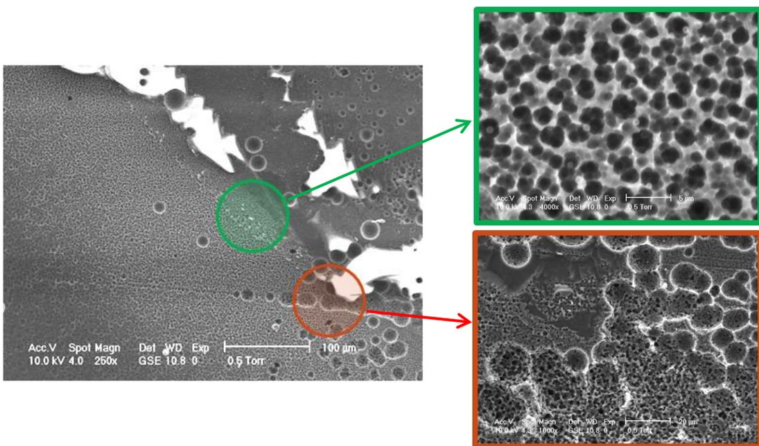
Figure 6: Surface morphology of a glass / carbon sample corroded at 1100°C.
