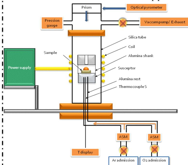
Figure 1: Cold wall set up
