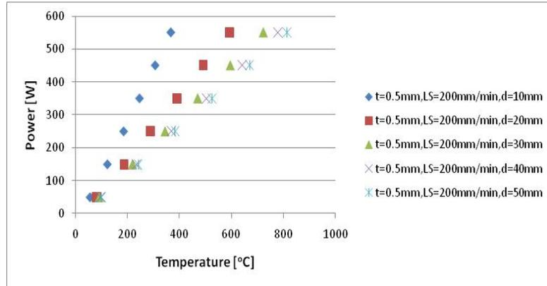
Figure 5: Welding temperature versus the laser power for different distance between the laser source and the material
