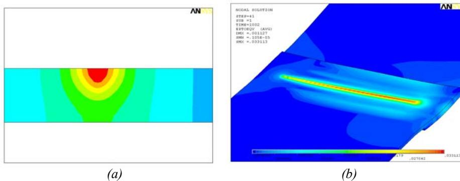
Figure 4: Calculated temperature distribution (a) and residual strains during the LTW process
