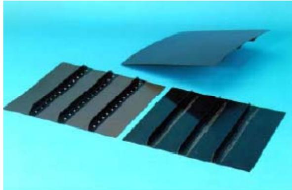
Figure 7: The panels with the riveted (on the left) and the laser welded (on the right) stiffeners
