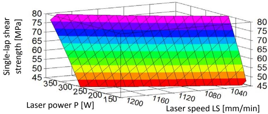
Figure 2: 3-dimensional plot combining the derived single-lap shear strength with the laser power  $P$  and the laser speed  $LS$
