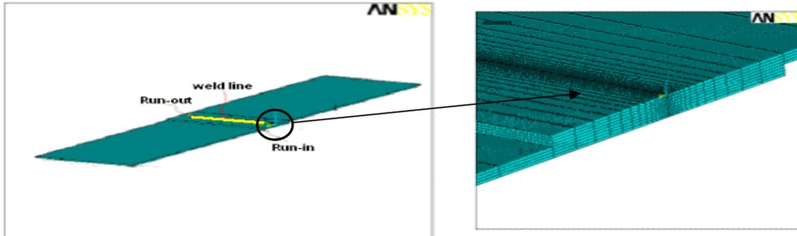
Figure 3: Finite element model created for the simulation of the LTW process
