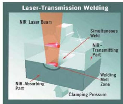
Figure 1: Laser Transmission Welding (LTW) technique [4]
