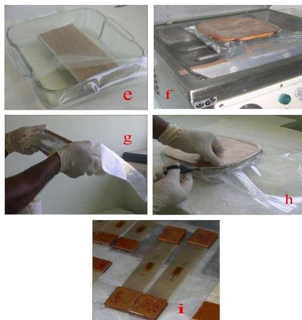
Figure 4: (e)-(h) Vacuum setting stages and 4(i) Sisal/Epoxy specimens.
