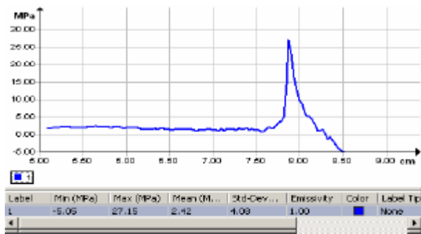
Figure 1: Stress field measurement from thermographic data.
