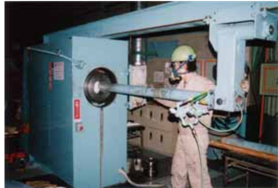
Fig.9: Inserting film bag role to centrifugal forming machine.
