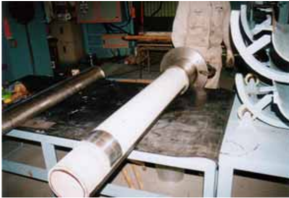
Fig.8: Inner rubber mould and separable outer metal mould.
