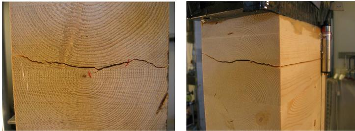
Figure 2: Crack path in unreinforced specimen
