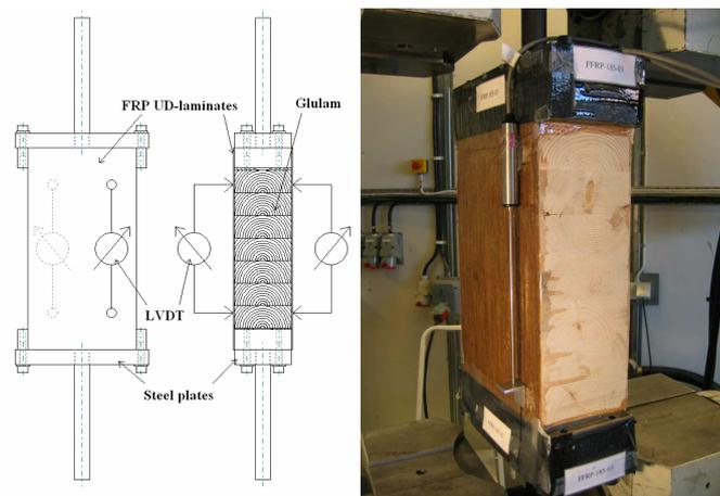
Figure 1: Test set-up for prismatic glulam specimen
