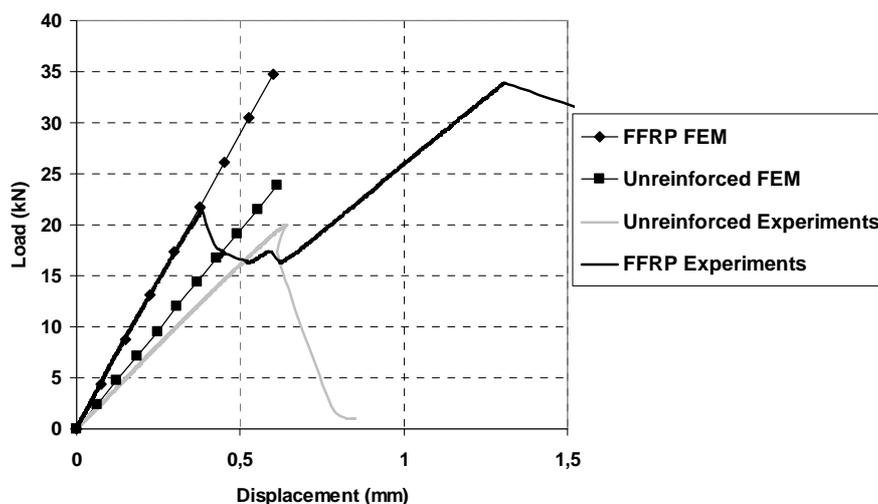
Figure 7: Load displacement curves for FFRP reinforced and unreinforced specimens
