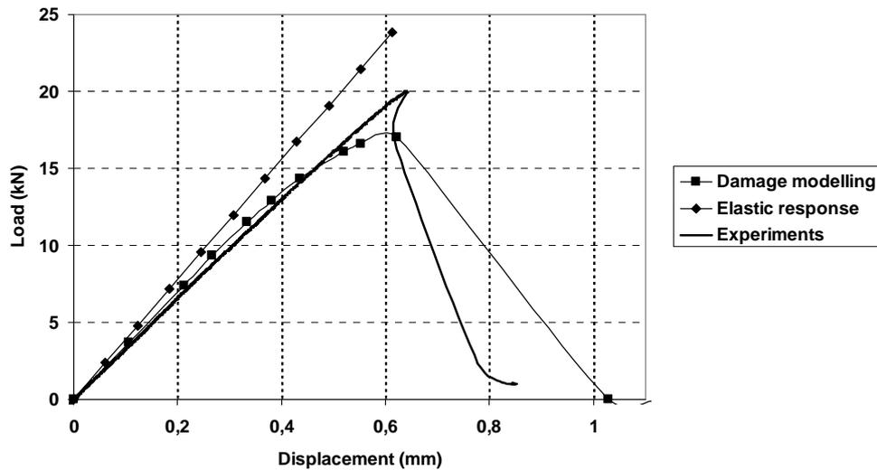
Figure 11: Load displacement curve for damage modelling of unreinforced specimen
