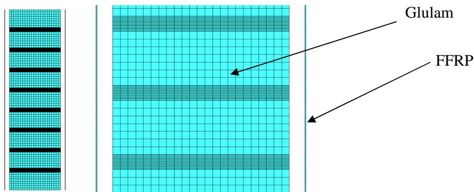
Figure 6: Assembly glulam-FFRP and mesh.
