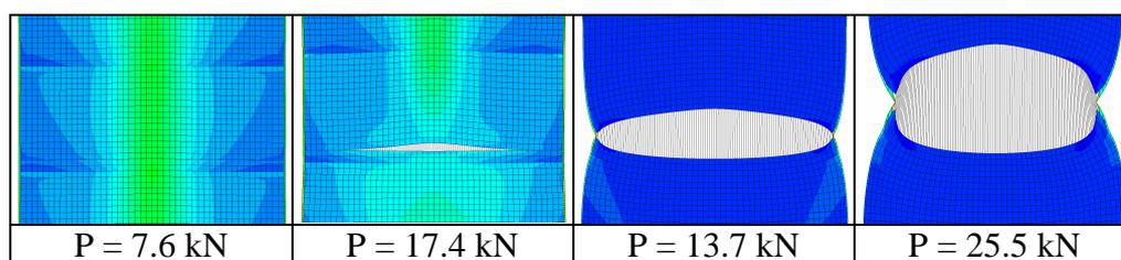
Figure 10: Crack propagation for FFRP reinforced specimens
