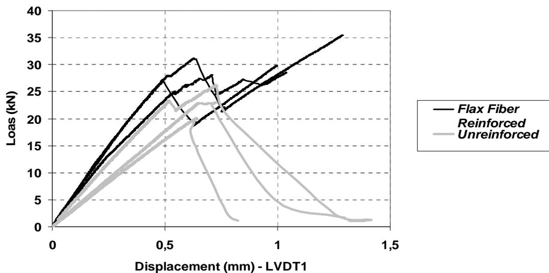
Figure 4: Load-displacement curves for experimental results
