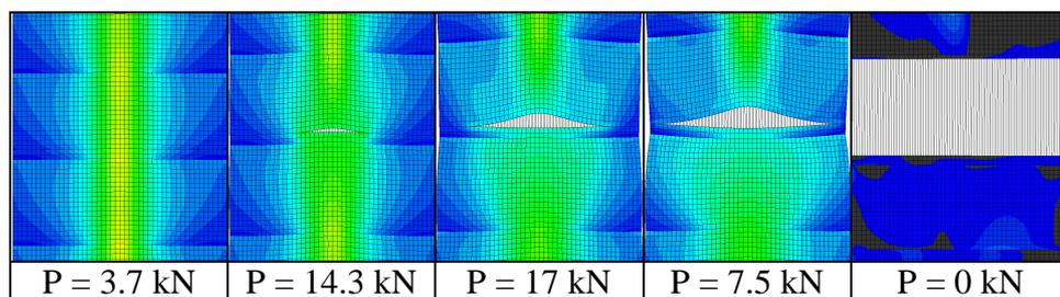
Figure 9: Crack propagation for unreinforced specimen.
