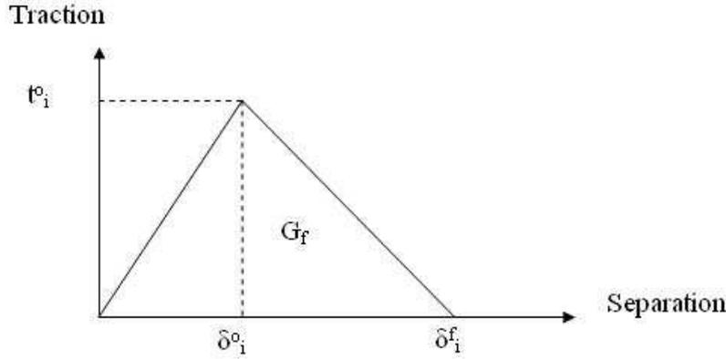
Figure 3: Traction separation response
