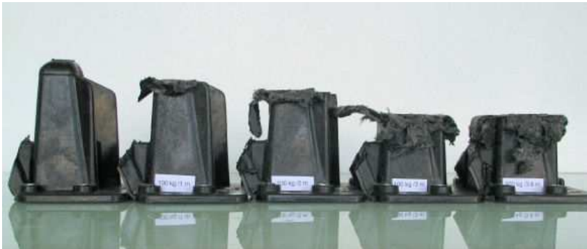
Fig. 6: evolution of damage due to impact (left to right: 0J, 1000J, 2000J, 3000J, 3600J)
