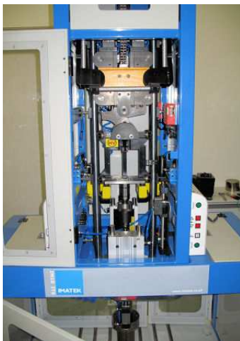
Fig. 5: ESTACA – LSM drop weight testing device (maximum capacity 4000J: 100kg and 4m)
