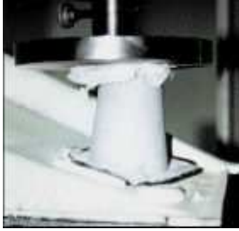
Fig. 1: MOZAIC quasi-static compression testing
