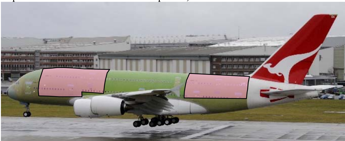
Figure 1: Application of GLARE ® on A380 (status 2008).
