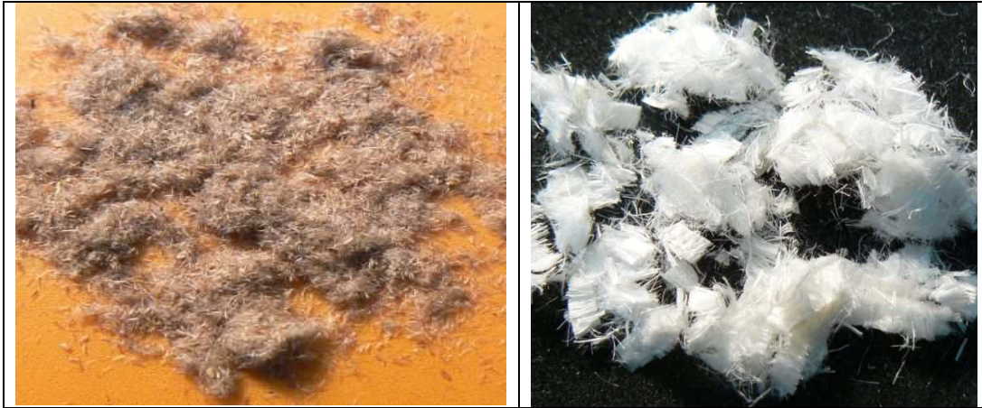
Figure 1: Flax fibres untreated (left) and bleached (right)
