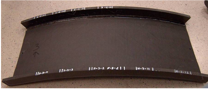
Figure 3 Flange section after demoulding
