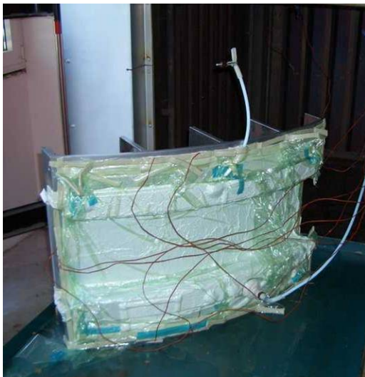
Figure 2 (a) Bagged flange on tool before resin injection (b) Sketch of flange cross-section
