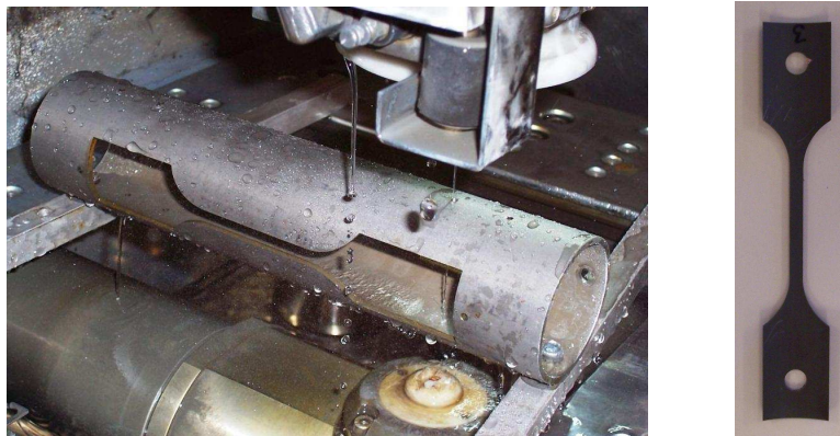
Figure 3: Machining of the specimens by wire EDM
