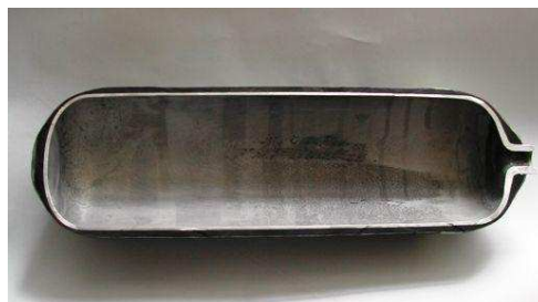
Figure 1: Section of a type III vessel
