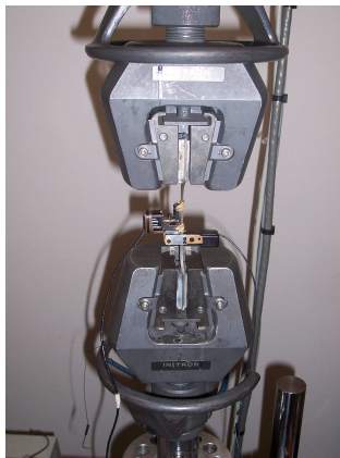
Figure 7: Set up and results of the fatigue tests with \frac{\sigma_{\min}}{\sigma_{\max}} = 0
