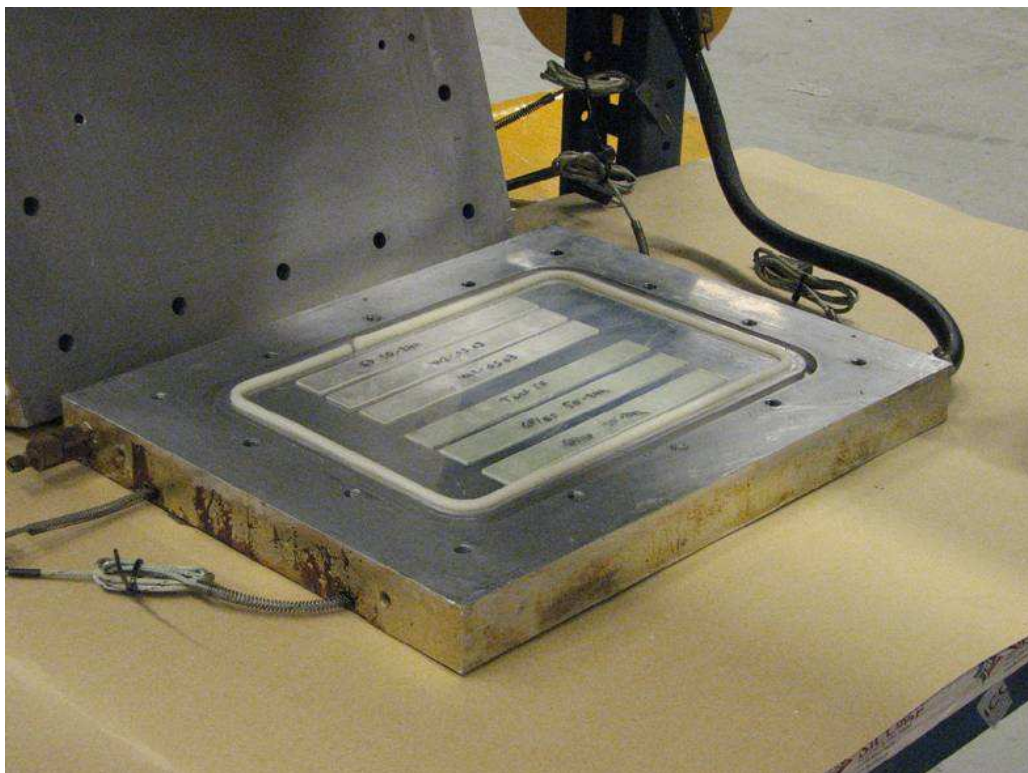
Figure 1. RTM mould and composite specimens after cutting-
