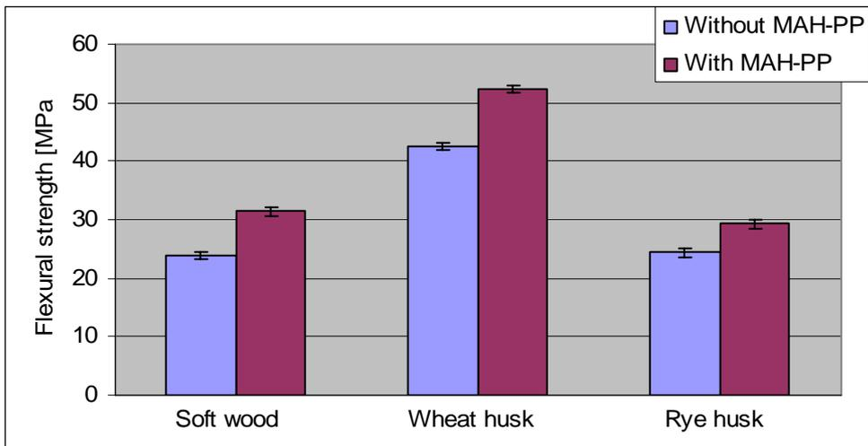
Figure4: Flexural strength of different fillers PP composites with and without MAH-PP.
