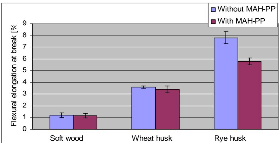
Figure5: Flexural elongation at break of different fillers PP composites with and without MAH-PP.
