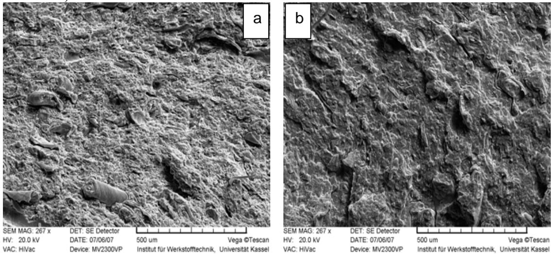
Figure10: SEM micrographs of rye husk- PP composites; a) without MAH-PP, b) with MAH-PP
