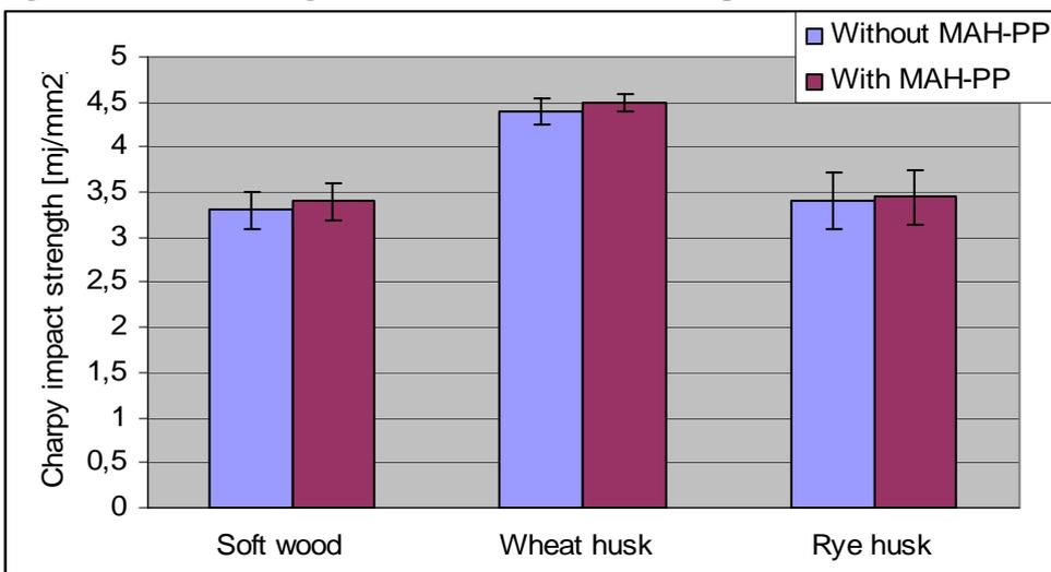
Figure8: Charpy impact strength of different fillers PP composites with and without MAH-PP.
