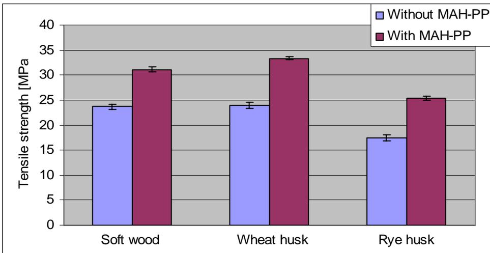
Figure7: Tensile strength of different fillers PP composites with and without MAH-PP.
