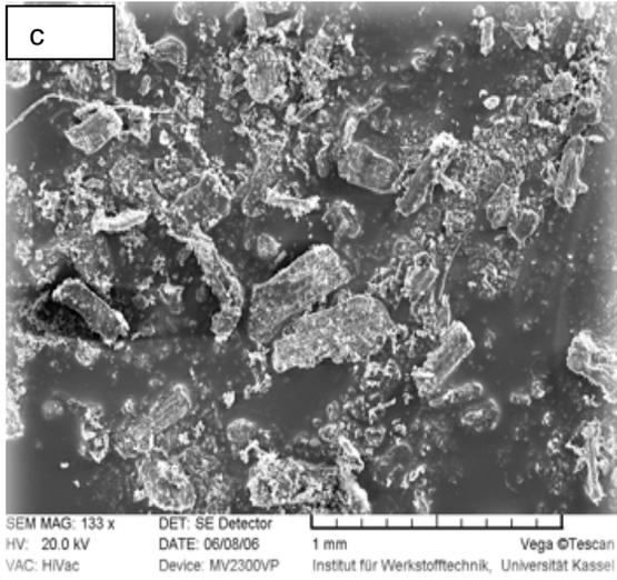
Figure1: SEM microgram of fibre geometry a) wheat husk, b) rye husk and c) soft wood.
