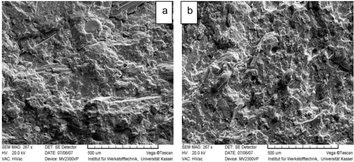
Figure9: SEM micrographs of wheat husk- PP composites; a) without MAH-PP, b) with MAH-PP
