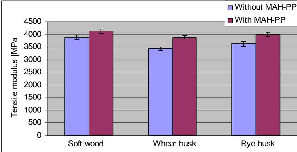
Figure6: Tensile modulus of different fillers PP composites with and without MAH-PP.
