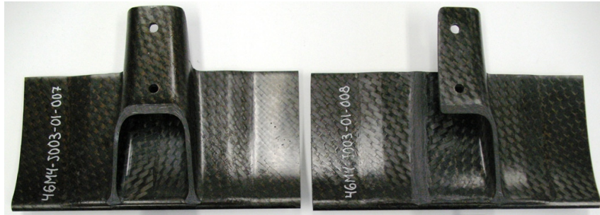
Figure 2: Prototype slats trimmed to obtain full and half bracket specimens in a middle configuration
