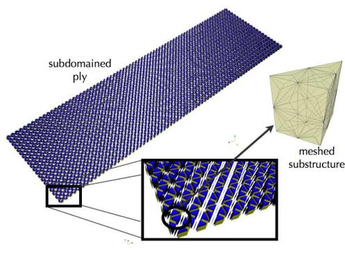
Figure 4: Illustration of the decomposition of a  $[\pm 45]_s$  ply;
