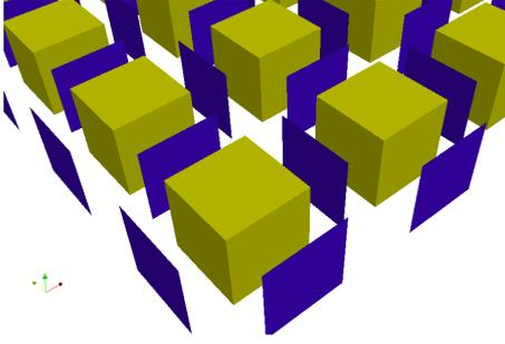
Figure 1: Repartition of fiber/matrix material and interfaces
