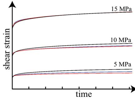
Figure 3: Comparison of the experiment (red), Schapery's linear model (black) and our model which includes the effective stress (blue)
