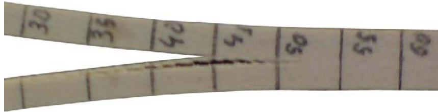
Figure 10: Branching phenomenon observed for “20 bars” and “30 bars” specimens
