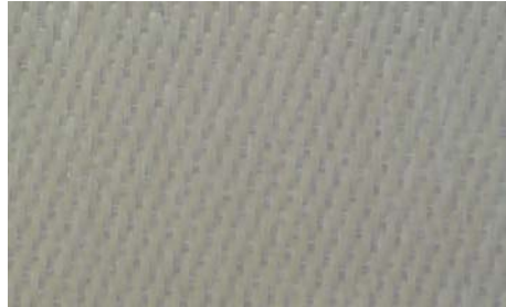
Figure 14: Rough delamination surface of a “10 bars” E-Glass reinforced specimen
