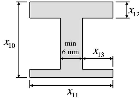
Figure 5: Stringer parameterization
