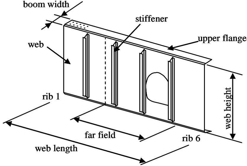
Figure 4: Outer side of the CWB rear spar
