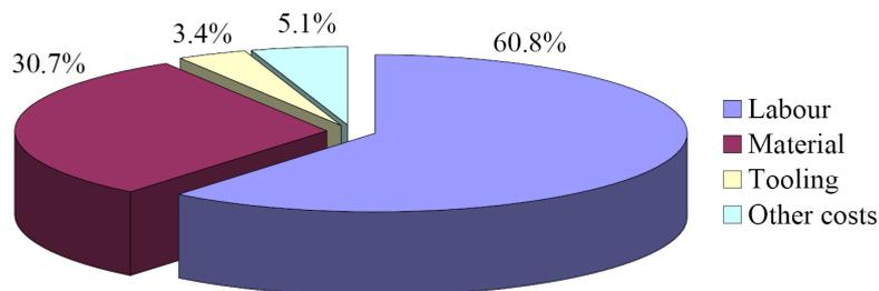
Figure 6: Cost allocation for the CWB rear spar at the *WP1500* test run optimum
