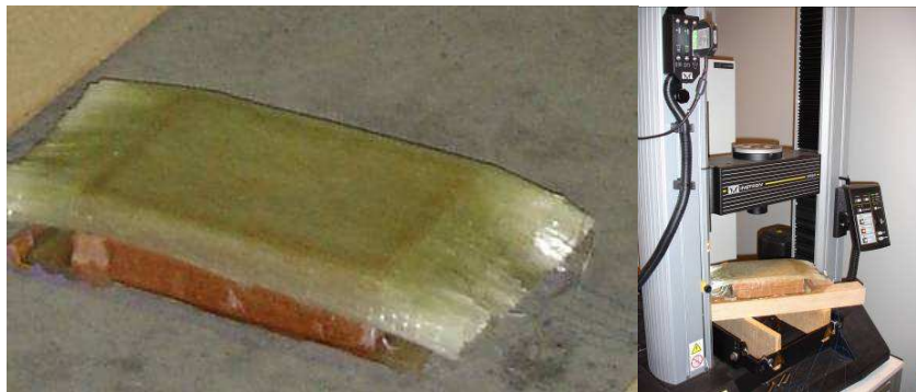
Figure 8 – Sample sandwich and testing machine
