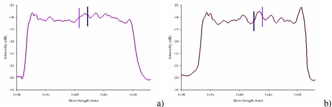
Figure 5: Reflected spectra from bonded joint with 3mm air defect a) under no load b) under 7 kN load.
