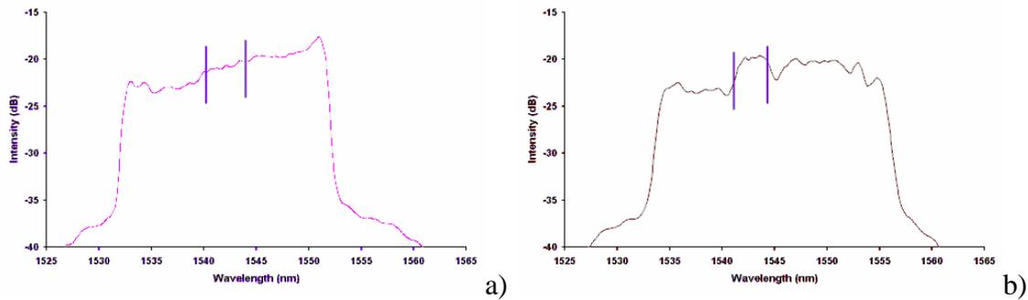
Figure 4: Reflected spectra from bonded joint with 12 mm PTFE defect a) unloaded; b) loaded to 9 kN.
