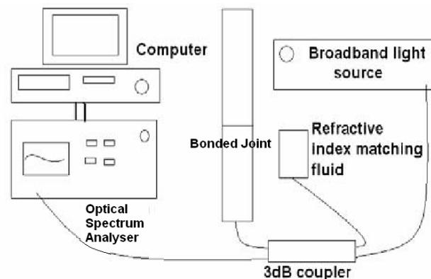
Figure 3: Schematic of the experimental arrangement
