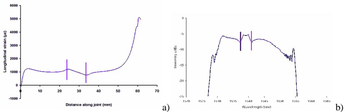
Figure 9: a) Longitudinal strain profile of joint with 10mm defect under a 7 kN load. b) Reflected spectrum predicted from strain profile.
