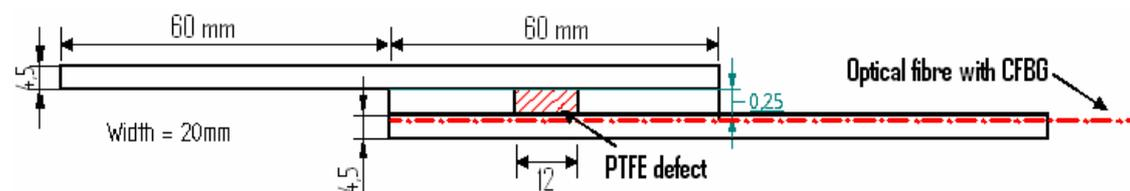
Figure 1: Geometry of bonded joint with PTFE defect.
