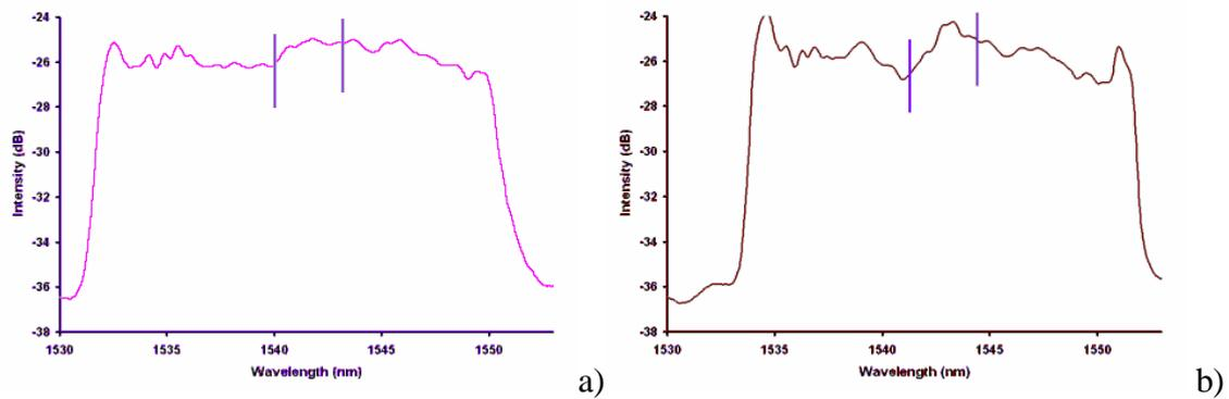
Figure 6: Reflected spectra from bonded joint with 10mm air defect a) under no load b) under 7 kN load.
