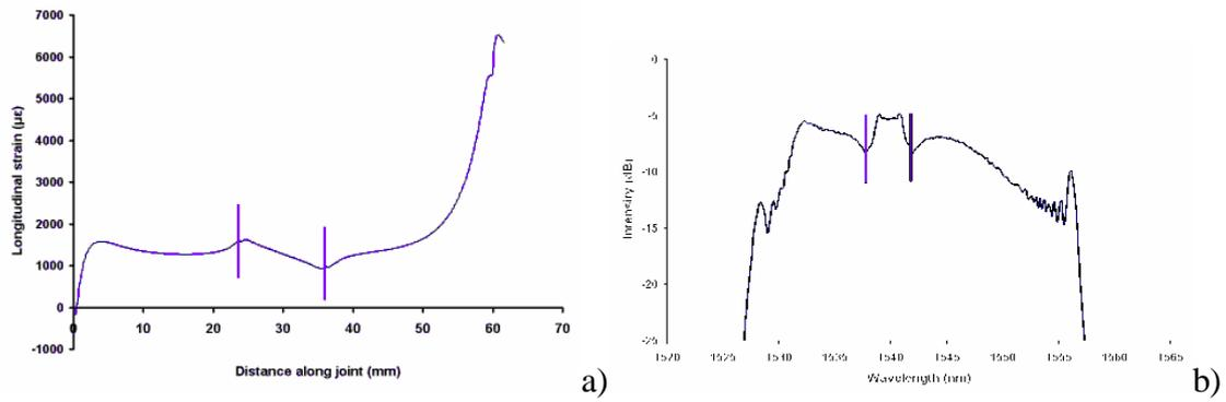
Figure 7: a) Longitudinal strain profile at the position of the core of the optical fibre for a joint with a central 12 mm defect under a 9 kN load. b) Reflected spectrum predicted from this strain profile.
