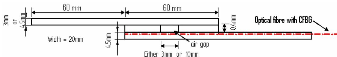
Figure 2: Geometry of bonded joint with air gap defect.
