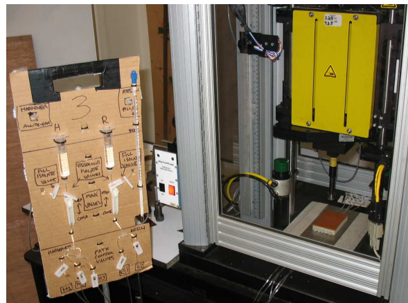
Figure 2. Photograph of specimen connected to resin and hardener supplies and positioned in preparation for drop-weight impact.
