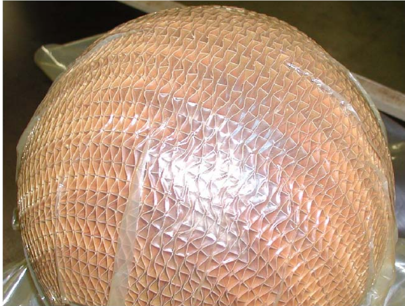
Figure 1. Sandwich cores with non-conventional cell shapes are flexible enough to be bent into complex shapes such as a sphere.
