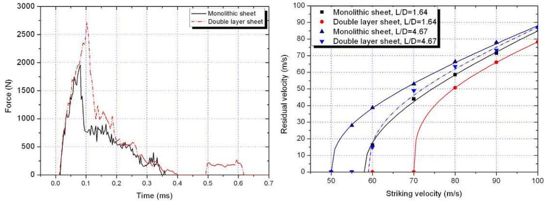
Figure 5 Calculated force on the flat nosed projectile ( $F_1$ ,  $L/D = 1.64$ ) during perforation of monolithic and layered sheets at an impact speed 80 m/s and an initial angle of obliquity of 30 degree
