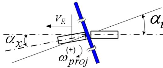
Figure 1 Schematic of oblique impact
