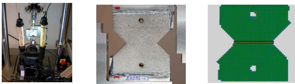
Figure 8: V-notched rail shear specimen: experimental set-up (left), specimen with black dots (centre), and ARAMIS sections defined (right).
