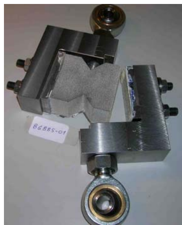
Figure 5: Initial tested V-notched rail shear specimen fractured at one of the corners (bottom right) with high peel stresses.
