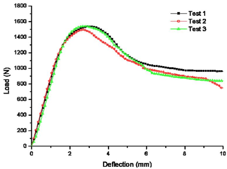
Figure 4: Load-deflection curves by 3-point bending tests
