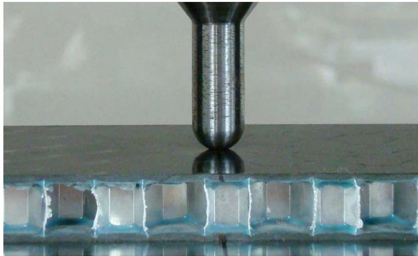
Figure 6: Quasi-static indentation test using UTM
