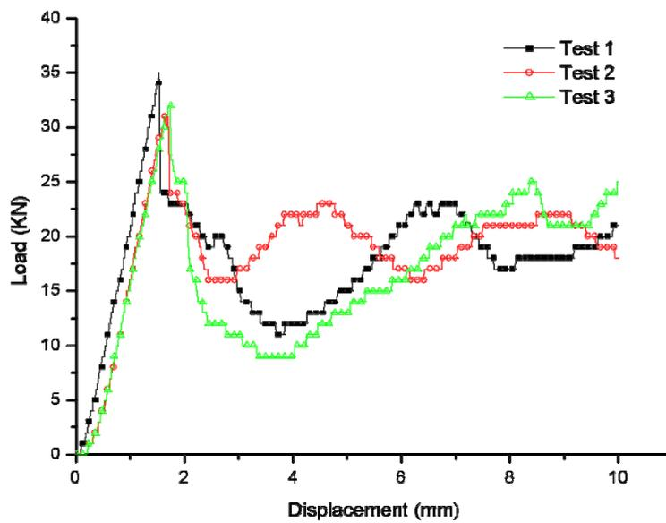
Figure 5: Load-displacement curves by compression tests
