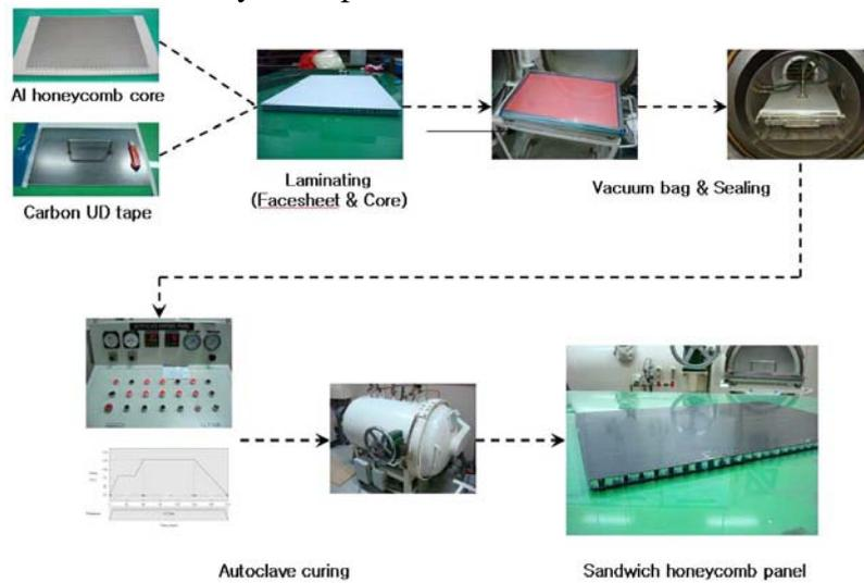
Figure 1: Co-curing process flow of Al honeycomb sandwich panel
