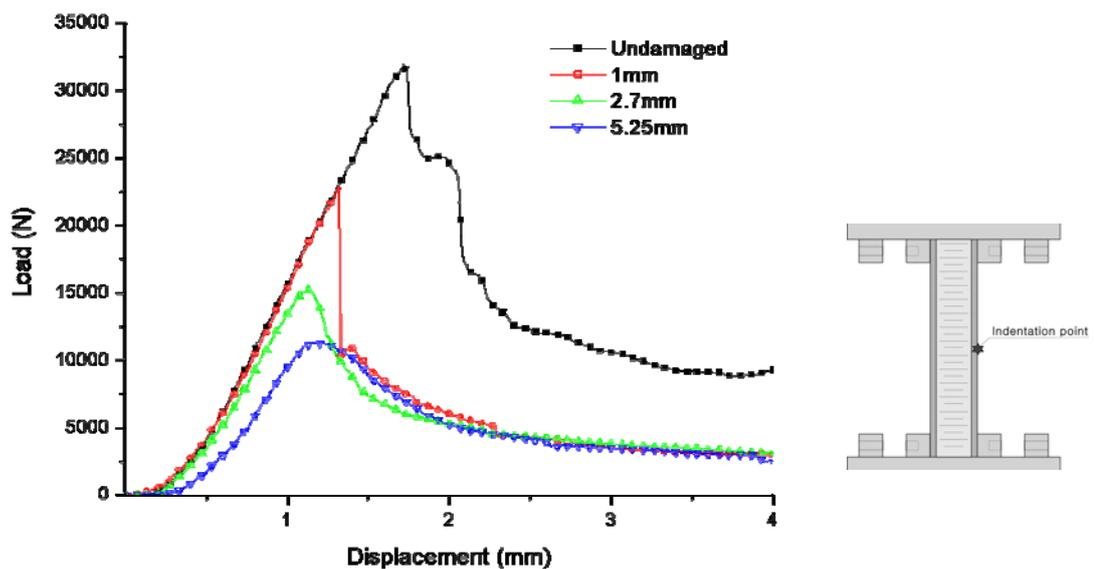
Figure 10: Load-displacement curves by compressive tests
