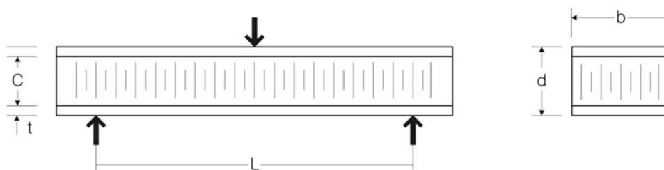
Figure 2: Schematic diagram of 3-point bending test
