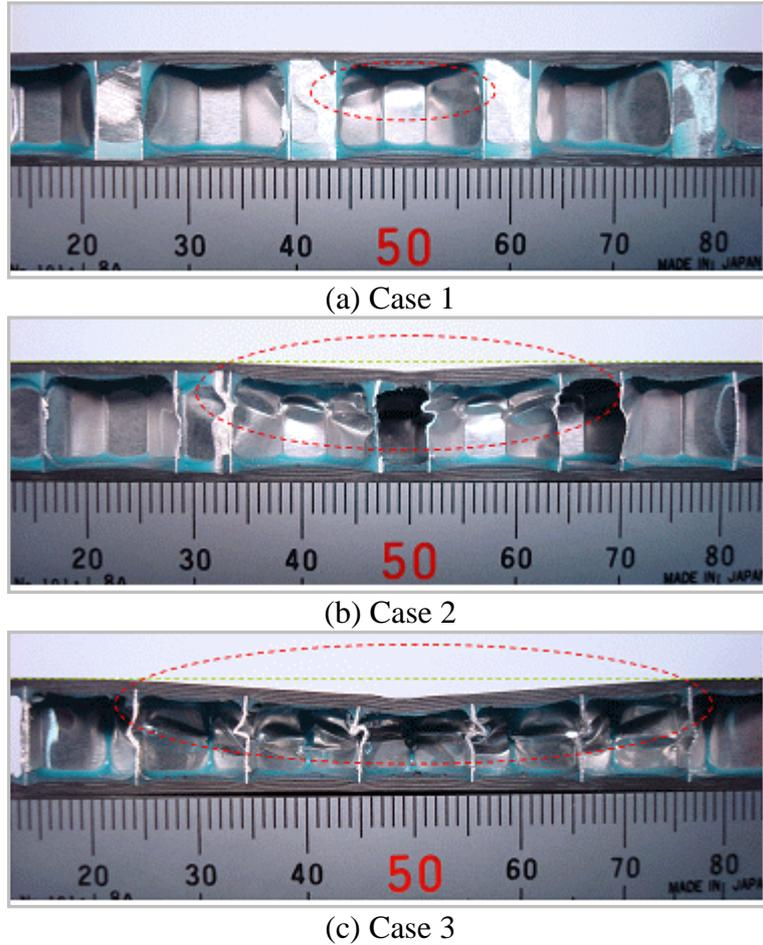
Figure 8: Cutting section of the indented specimen
