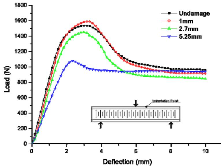
Figure 9: Load-deflection curves by 3-point bending tests
