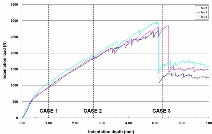
Figure 7: Load-indentation depth of the quasi-static indentation
