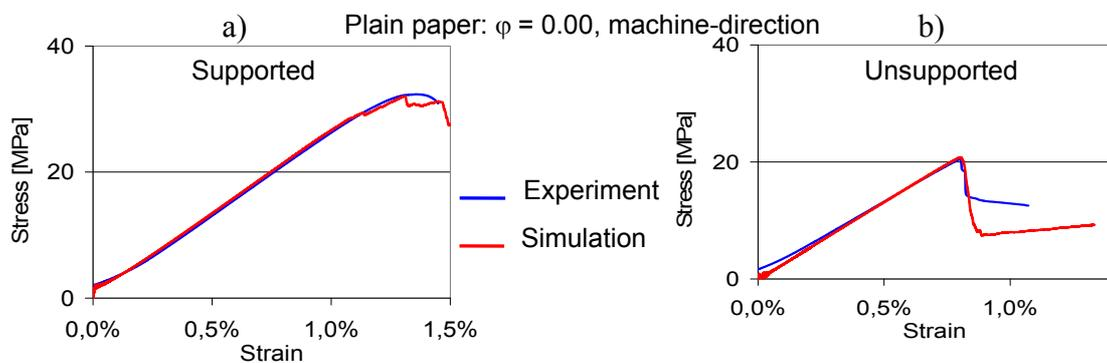
Figure 11: Validation of simulation models for compressive loading: a) supported specimen, b) unsupported specimen
