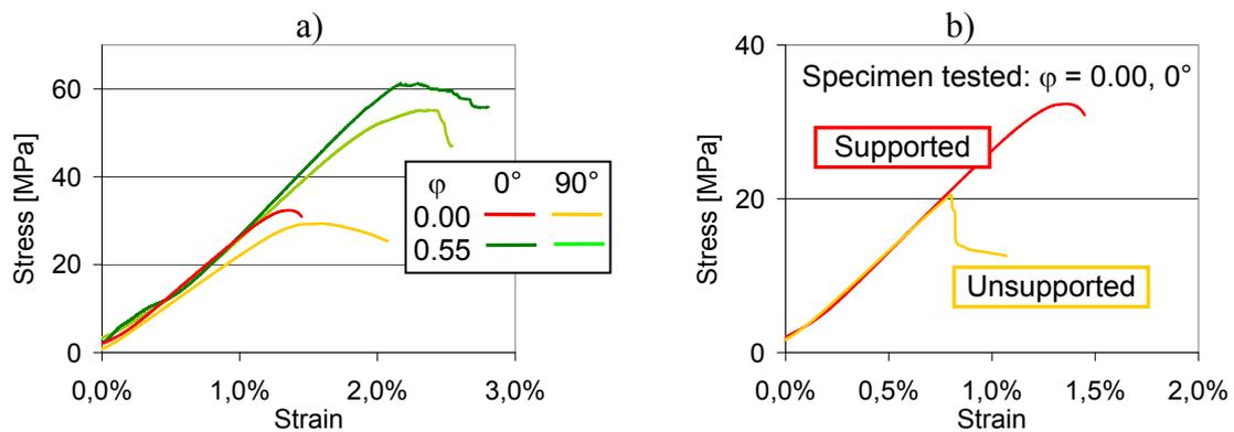
Figure 8: a) Stress strain results of test utilizing the modified compression test setup, b) Material characteristics for supported and unsupported specimens
