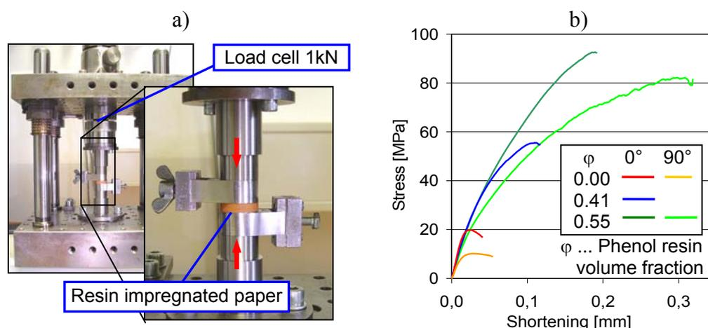
Figure 6: a) Compression test fixture, b) Example of the obtained compressive material characteristics for plain and impregnated paper
