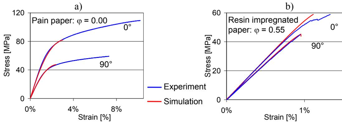
Figure 9: Validation of simulation models for tensile loading: a) plain paper, b) phenol resin impregnated paper
