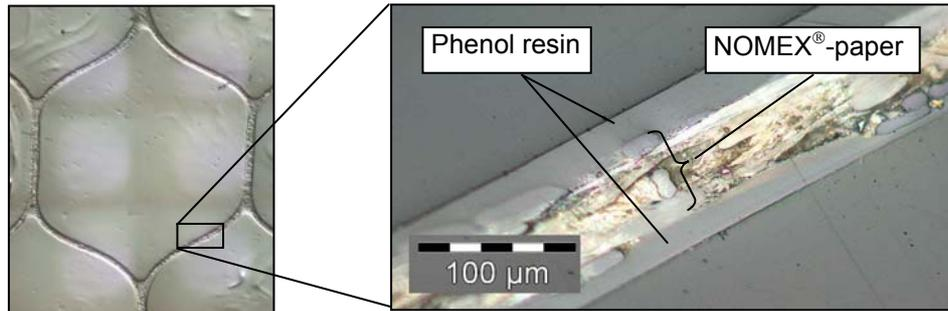
Figure 3: Micrographs of 4.8-64 NOMEX<sup>®</sup>-honeycomb cell and single cell wall
