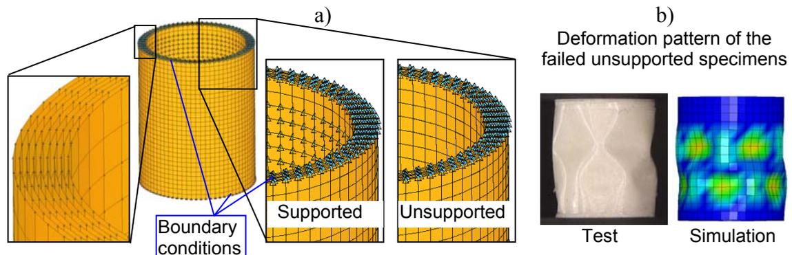
Figure 10: Simulation of the compressive loading: a) finite element model of the coiled paper specimen, b) failure of unsupported specimen
