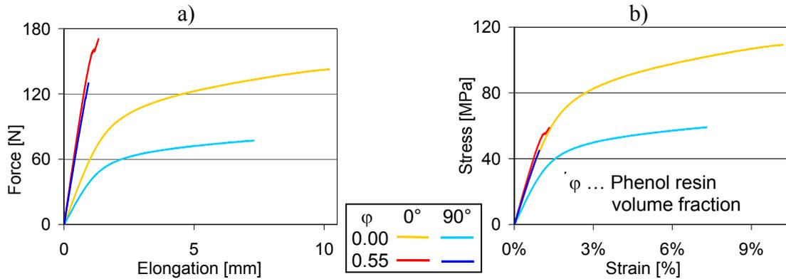
Figure 4: a) Recorded load-elongation functions of different papers and directions, b) Stress-strain function of the investigated papers
