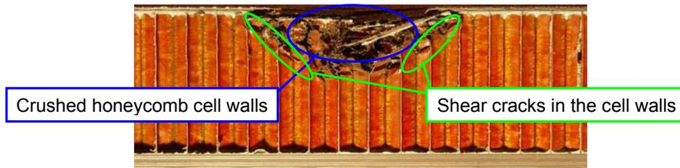
Figure 1: Impact damage of a non-metallic honeycomb sandwich
