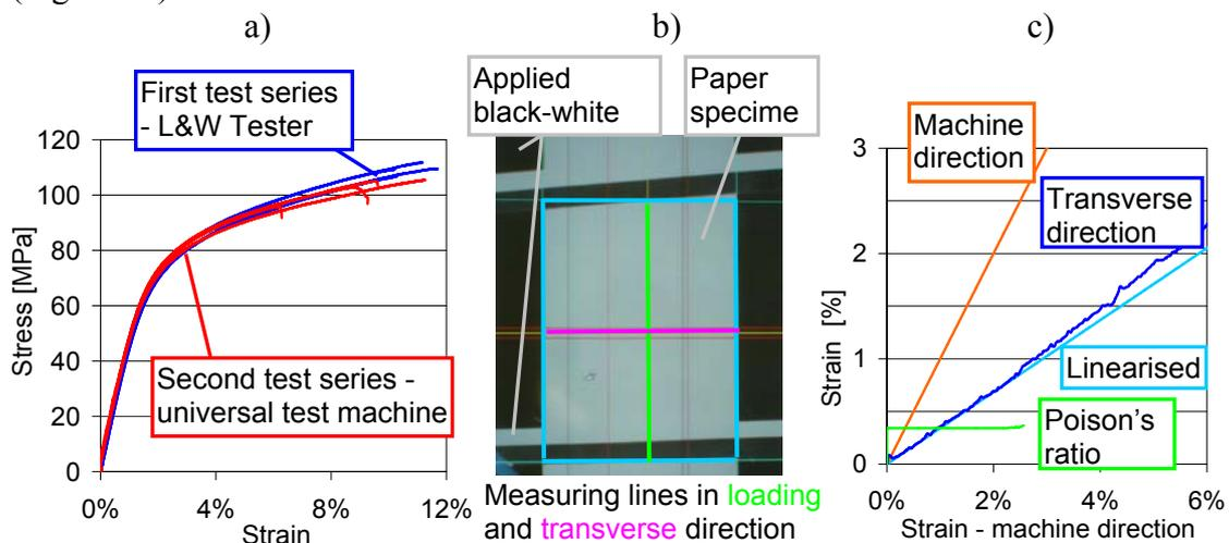
Figure 5: a) Stress-strain function of the two test series, b) Measurement field of the video extensometer, c) Measured strains and calculated Poisson's ratio
