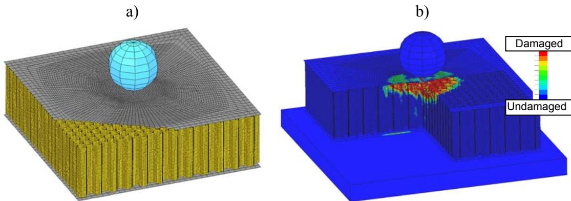
Figure 12: a) Impact simulation model, b) Cross-sectional view of damaged sandwich structure (here: 8J Impact)
