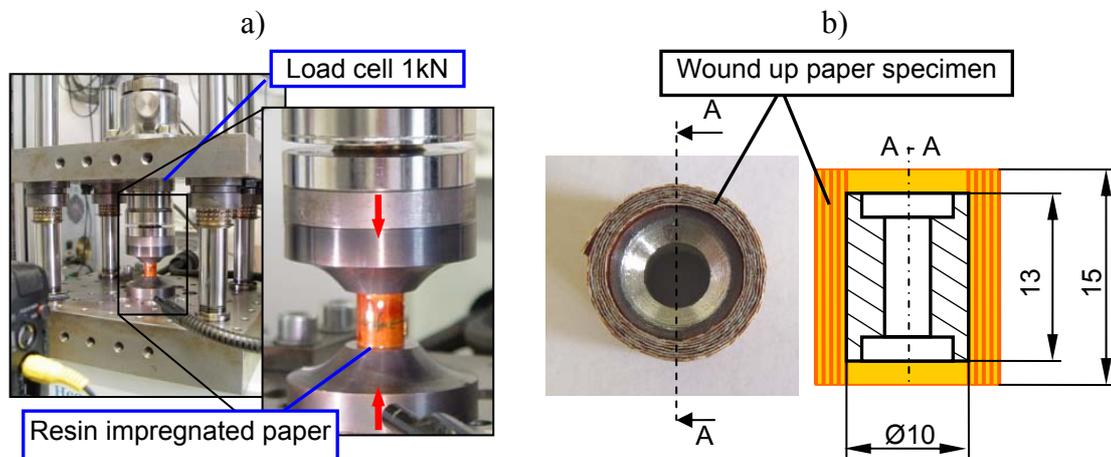
Figure 7: a) Modified compression test setup, b) Prepared paper specimen
