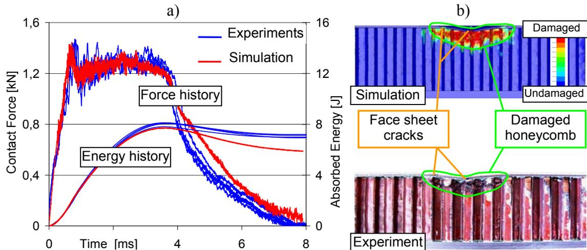
Figure 13: a) Force and energy plots of experiments and simulation (here 8J impact),
