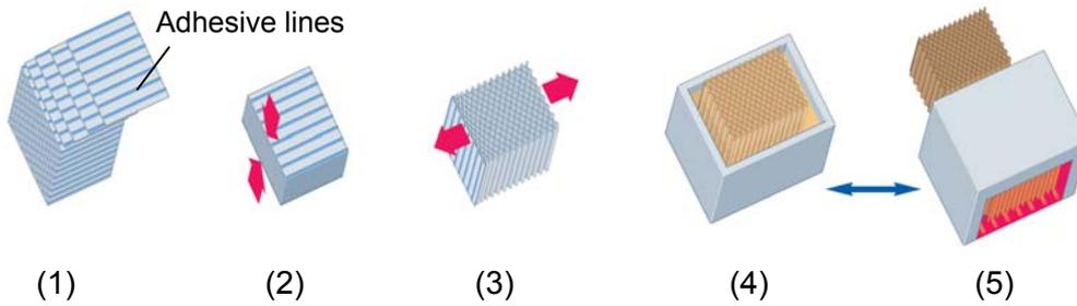
Figure 2: Manufacturing process of phenol resin impregnated honeycomb core [8]
