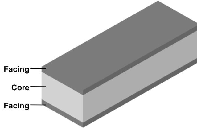
Figure 1: A typical sandwich construction.
