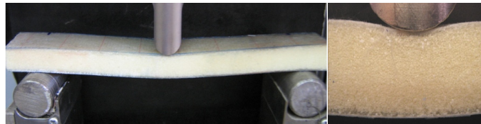
Fig 10 Three point bending in sandwich beam of A
