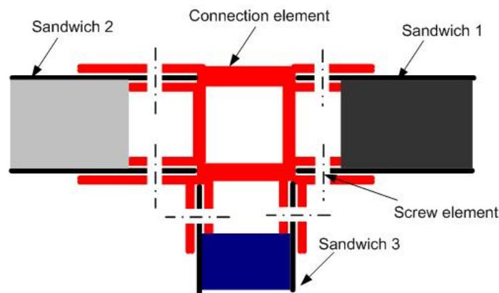
Figure 5: Principle sketch of a T-joint connecting 3 different sandwich materials
