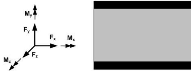
Figure 2: General forces and moments in a sandwich element
