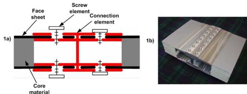
Figure 1: Principle solution and a functional model
