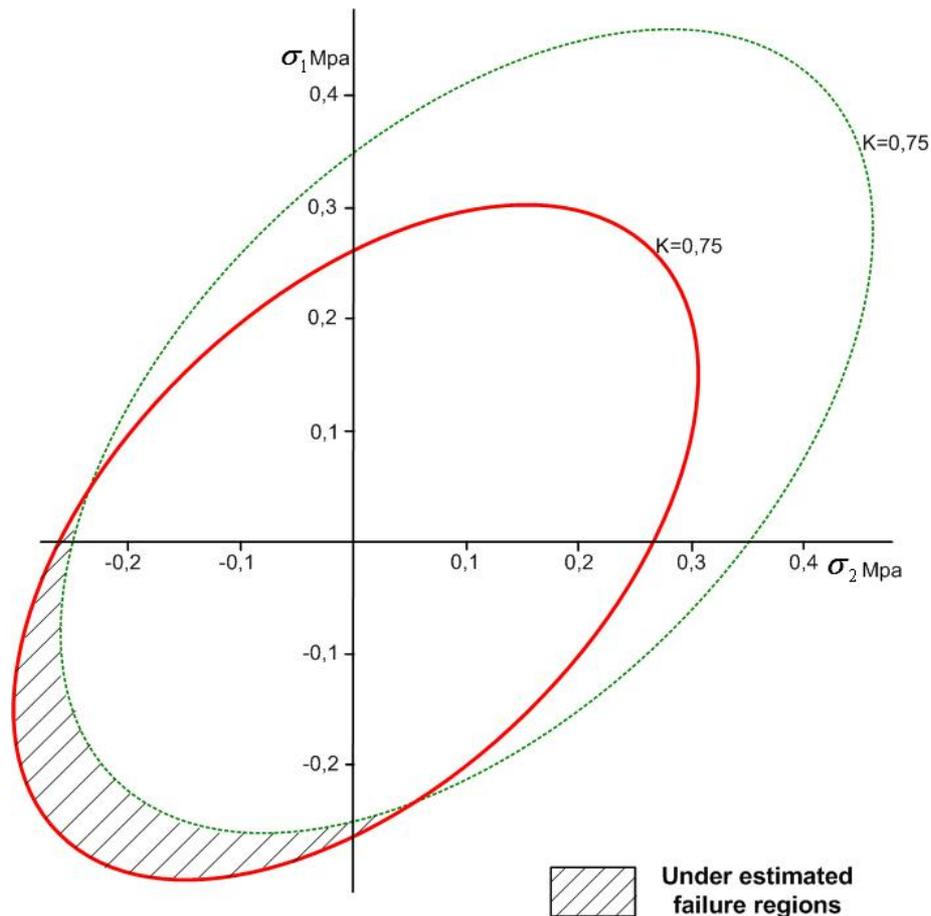
Figure 3: 2D illustration of failure criteria- a comparison
