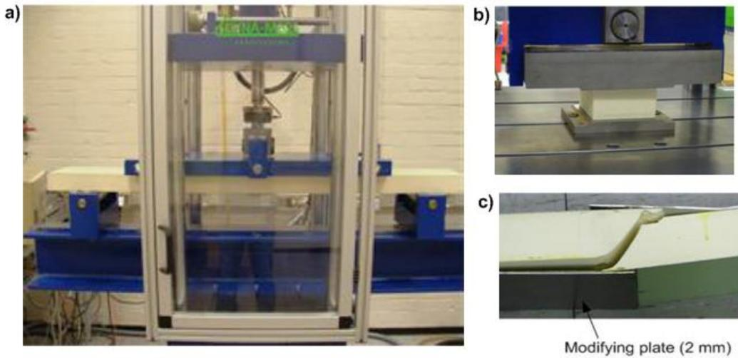
Figure 6a): four-point bending; Figure 6b): Compressive test; Figure 6c): Shear failure
