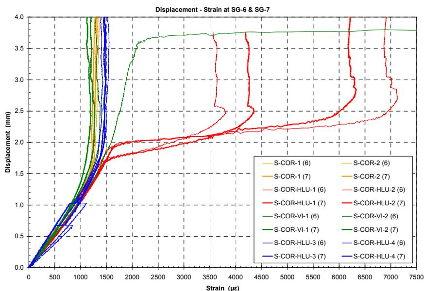
Figure 6: Strains at SG-6 and SG-7 versus applied displacement.
