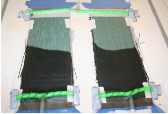
Figure 3: Vacuum infusion of specimens S-COR-VI-1 & 2.
