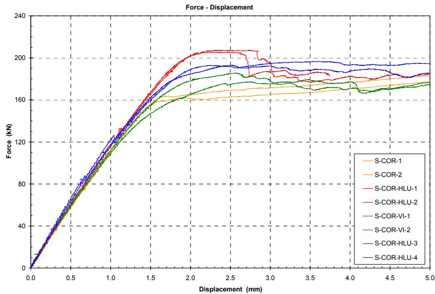
Figure 4: Specimens' elongation versus applied load.
