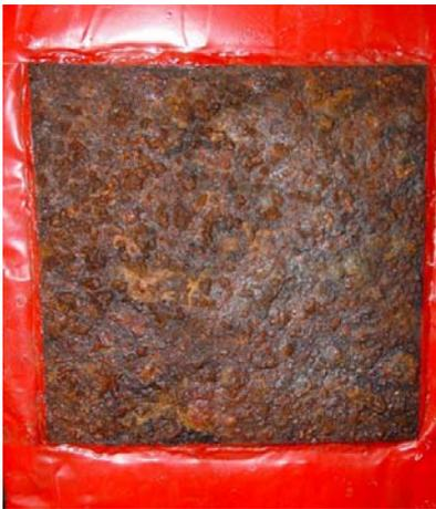
Figure 2: Specimen S-COR-VI-1 after its removal from the salt spray chamber.
