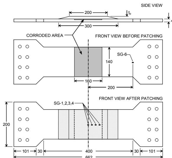
Figure 1: Specimen geometry.
