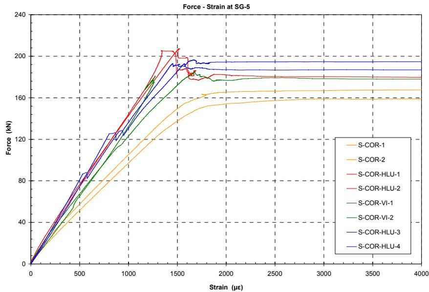
Figure 5: Strains at SG-5 versus applied load.
