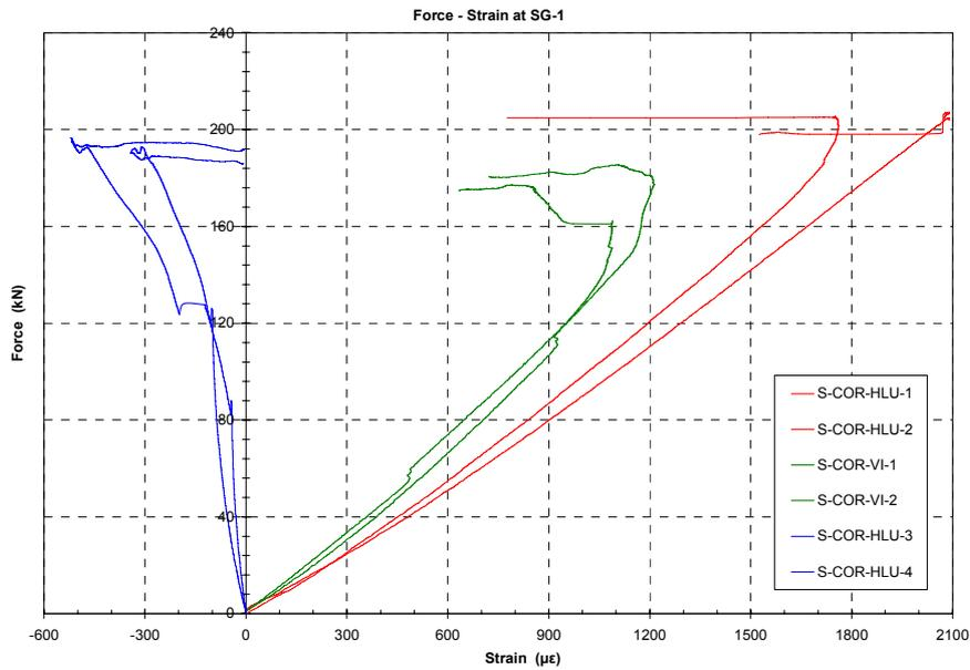
Figure 7: Strains at SG-1 versus applied load.
