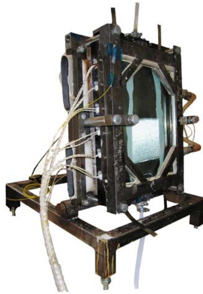
Figure 2. Transparent mould used for the RTM injections
