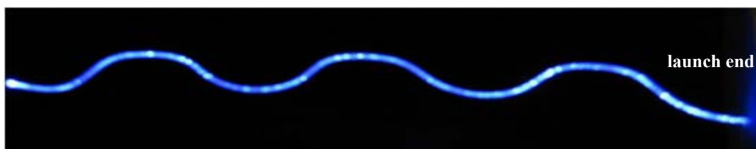
Figure 9: Fibre 3, treated with silica particles, twelve bends with 17 mm radius; bright spots indicate emission at scattering particles.
