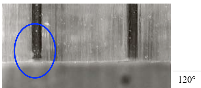
Figure 6 : Close up of a photograph taken of a debonded wire edge at 120°C
