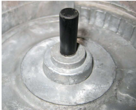
Fig. 1. Composite rod imbedded in pressure die casted aluminium.
