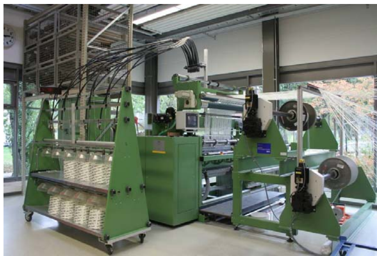
Figure 2: Stitch bonding machine Karl Mayer Malimo 14022 P2-2S.
