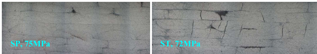
Fig. 2: NCF laminates tested in compression. Tests were interrupted before final failure.
