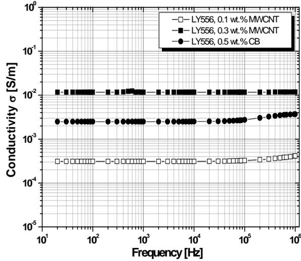
Fig. 1: Conductivity values of the nanocomposites.
