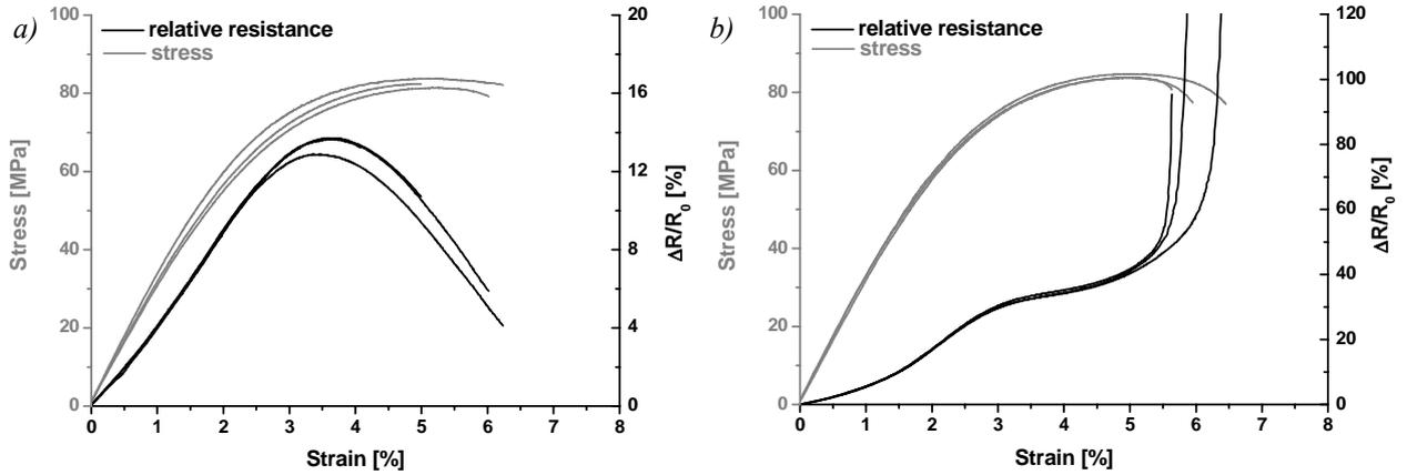
Fig. 2: Stress-strain and resistance-strain curves of different epoxy based nanocomposites: a) 0.1 wt.% MWCNTs, b) 0.5 wt.% carbon black.
