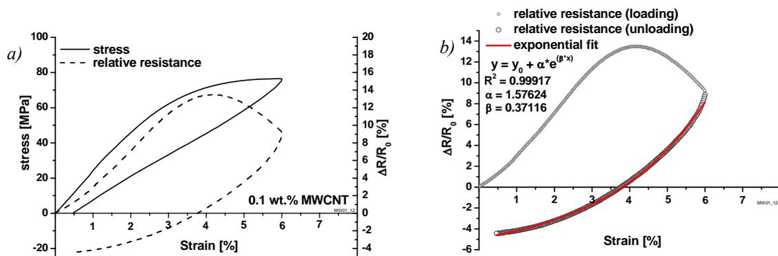
Fig. 4: a) Stress-strain curve and corresponding resistance change for loading and unloading of a 0.1 wt.% MWCNT specimen, b) exponential approximation of the resistance change during unloading.
