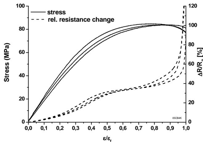
Fig. 5: Stress and relative resistance change vs. normalised strain  $\varepsilon/\varepsilon_f$  for the 0.5 wt% CB nanocomposites.
