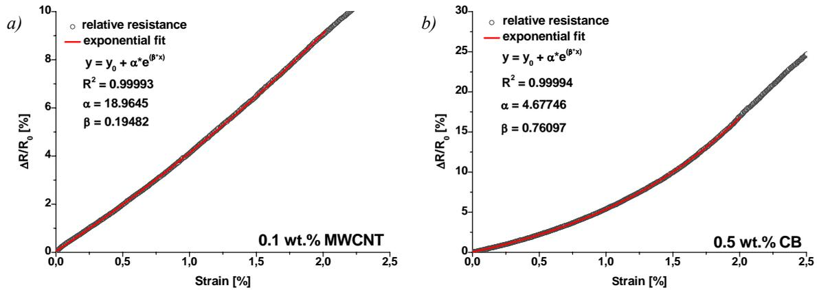
Fig. 3: Resistance-strain curves and exponential fitting functions of different epoxy based nanocomposites: a) 0.1 wt.% MWCNTs, b) 0.5 wt.% carbon black.
