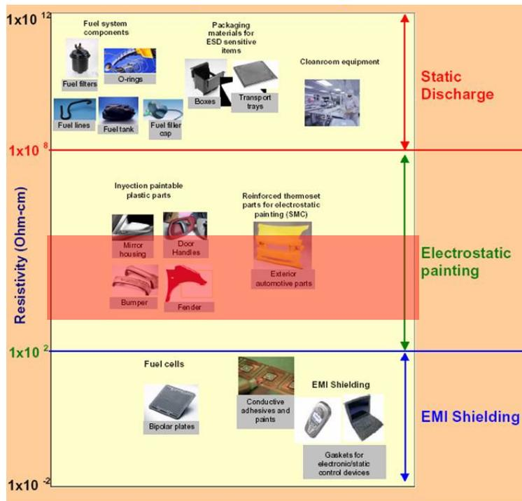
Figure 7. Composites application as a function of their electrical resistivity and the range of the studied composites values (marked in red).
