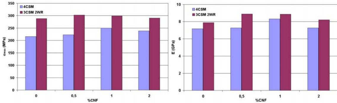
Figure 2. Flexural strength ( $\sigma_{max}$ ) and modulus of elasticity in bending (E) obtained results for composites prepared by the Hand Lay-up method.
