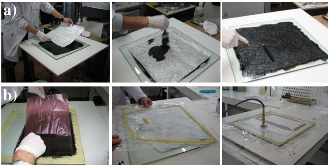
Figure 1. a) Hand lay-up method steps and b) vacuum bag method extra steps.
