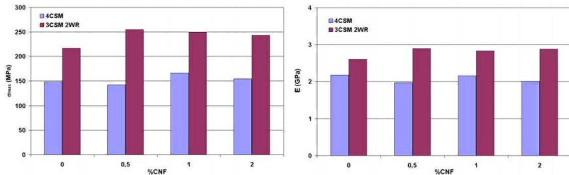
Figure 5. Ultimate Tensile Strength ( $\sigma_{\max}$ ) and Young's modulus (E) obtained results for composites prepared by the Vacuum Bag method.
