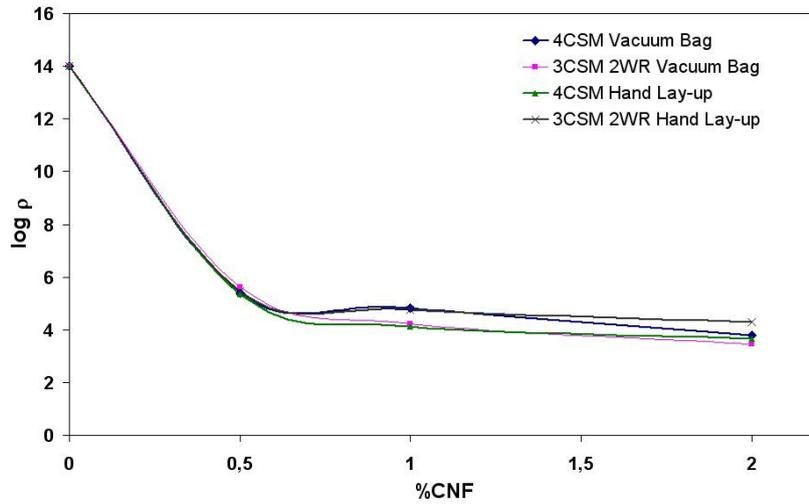
Figure 6. Log  $\rho$  ( $\Omega\cdot\text{cm}$ ) as a function of the %CNF in the matrix of the composites.
