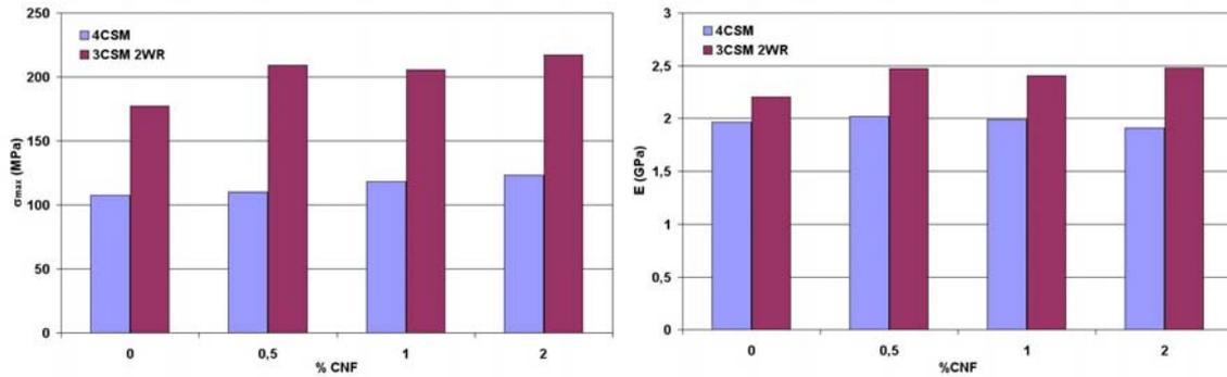
Figure 4. Ultimate Tensile Strength ( $\sigma_{\max}$ ) and Young's modulus (E) obtained results for composites prepared by the Hand Lay-up method.
