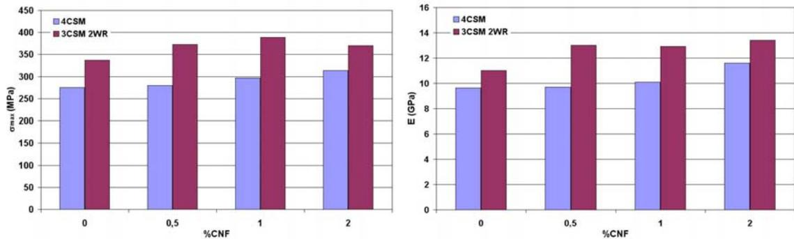
Figure 3. Flexural strength ( $\sigma_{max}$ ) and modulus of elasticity in bending (E) obtained results for composites prepared by the Vacuum Bag method.
