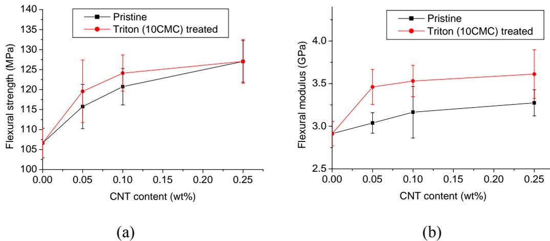
Fig. 6 (a) Flexural strength and (b) flexural modulus of CNT/epoxy nanocomposites with and without Triton (10 CMC) treatment
