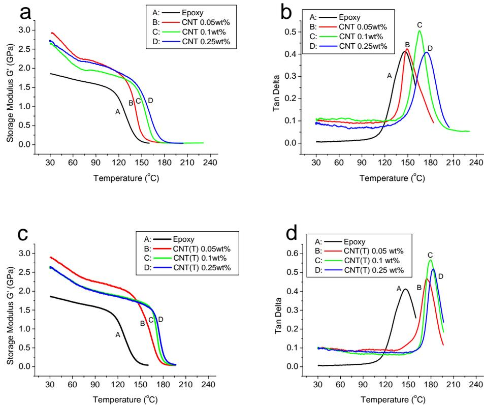
Fig. 4 (a) Storage modulus ( $G'$ ) and (b)  $\tan \delta$  of pristine CNT/epoxy nanocomposites; (c) storage modulus ( $G'$ ) and (d)  $\tan \delta$  of 10 CMC Triton treated CNT/epoxy nanocomposites as a function of temperature
