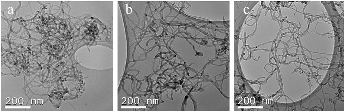
Fig. 3 TEM images of (a) pristine; (b) Triton X-100 (1 CMC) treated; and (c) Triton X-100 (10 CMC) treated CNTs
