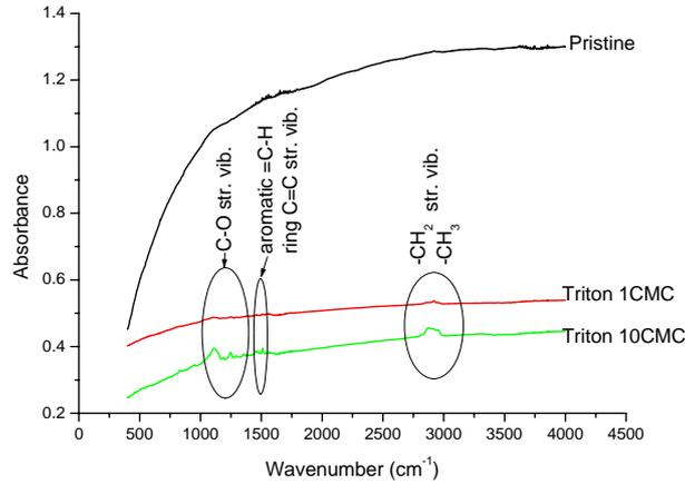
Fig. 2 FTIR spectra of CNTs with and without Triton treatment
