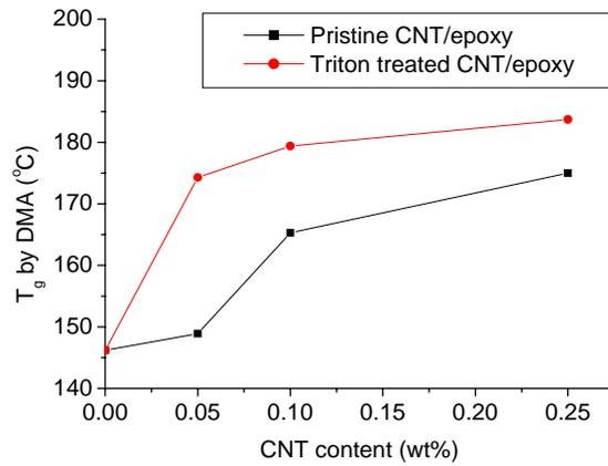
Fig. 5 Glass transition temperature ( $T_g$ ) of CNT/epoxy nanocomposites
