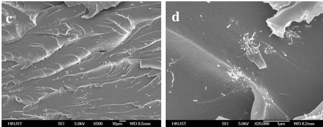
Fig. 8 SEM images of impact fracture surfaces of (a,b) pristine; (c,d) Triton (10 CMC) treated CNT/epoxy nanocomposites
