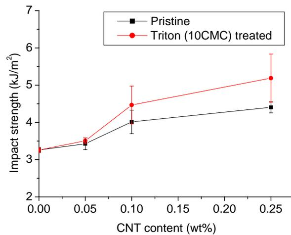
Fig. 7 Impact fracture toughness of CNT/epoxy nanocomposites with and without Triton (10 CMC) treatment
