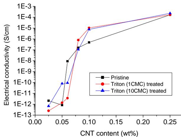
Fig. 9 Electrical conductivity of CNT/epoxy nanocomposites with and without Triton treatment.
