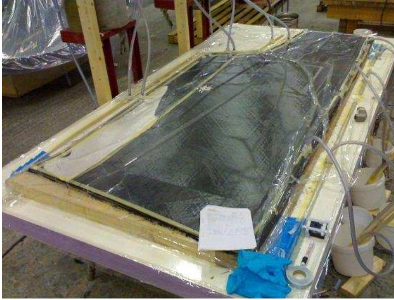
Picture 2 Undergoing infusion process of a sandwich panel
