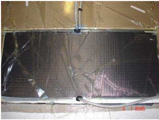
Picture 1 Resin infusion of single skin panel
