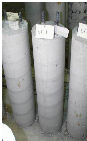
Figure 1: Photograph of selected cylindrical specimens showing the metal cages [1].
