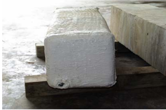
Figure 2: Photograph of a wrapped rectangular specimen during a drying period [3].
