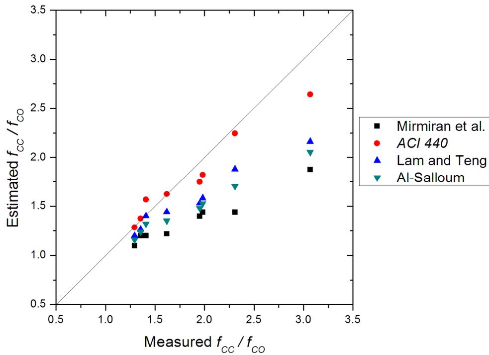
Figure 6: Comparison of the measured and estimated values of the normalized compressive strength of the confined square concrete specimens. Solid line – ideal correspondence.
