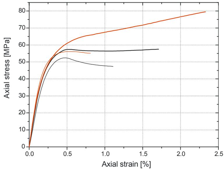
Figure 3: Axial stress-strain curves of the confined square concrete columns (concrete batch II). Thin line – 2 layers of the CFRP, thick line – 4 layers of the CFRP. Black line –  $r=15$  mm, red line –  $r=30$  mm.
