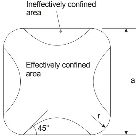
Figure 4: Cross-section of the square concrete column.
