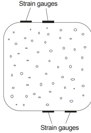
Figure 1: Arrangement of the strain gauges in the hoop direction.
