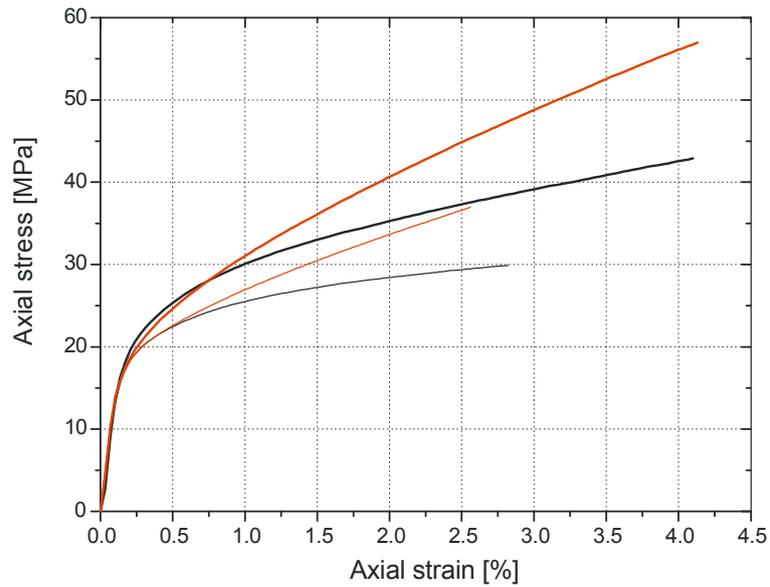
Figure 2: Axial stress-strain curves of the confined square concrete columns (concrete batch I). Thin line – 2 layers of the CFRP, thick line – 4 layers of the CFRP. Black line –  $r=15$  mm, red line –  $r=30$  mm.
