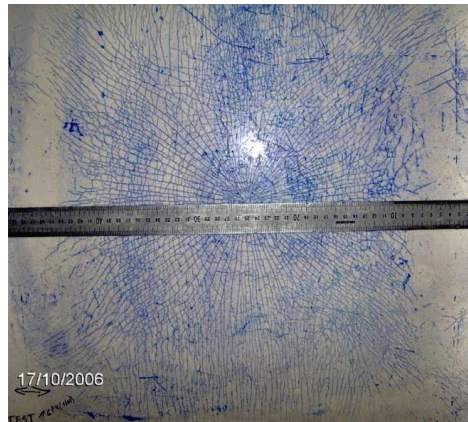
Figure 2: Crack pattern under low-speed impact and directions of principle stresses under static loading.
