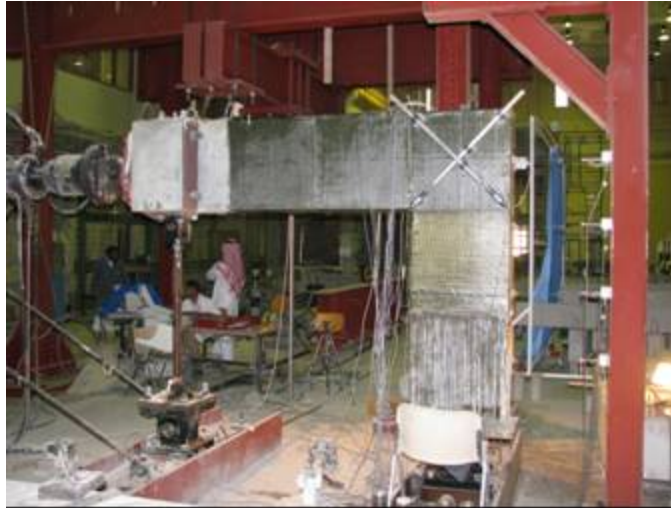
Figure 3: FRP scheme, instrumentation and test setup.
