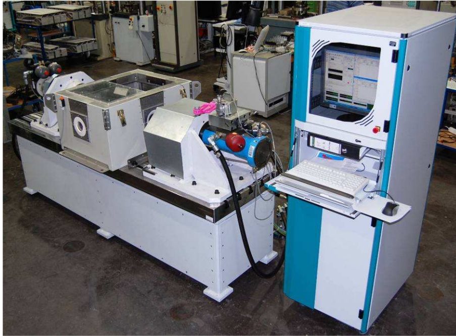
Figure 2: Servo-hydraulic testing machine used to test the V-notched specimens
