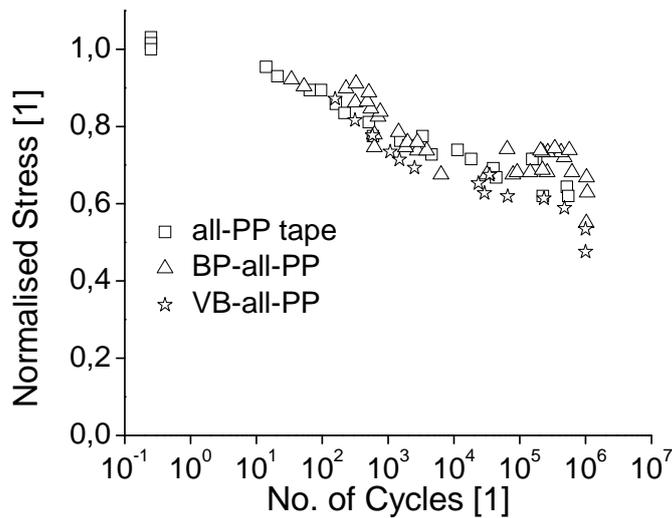
Figure 3. Normalised stress ( $\sigma/\sigma_0$ ) as a function of the number of cycles to failure, of PP-tapes, BP-, VB-all-PP woven composites comparing the fatigue response and the damage development of these materials.  $\sigma_0$  corresponds to the UTS of respective material.
