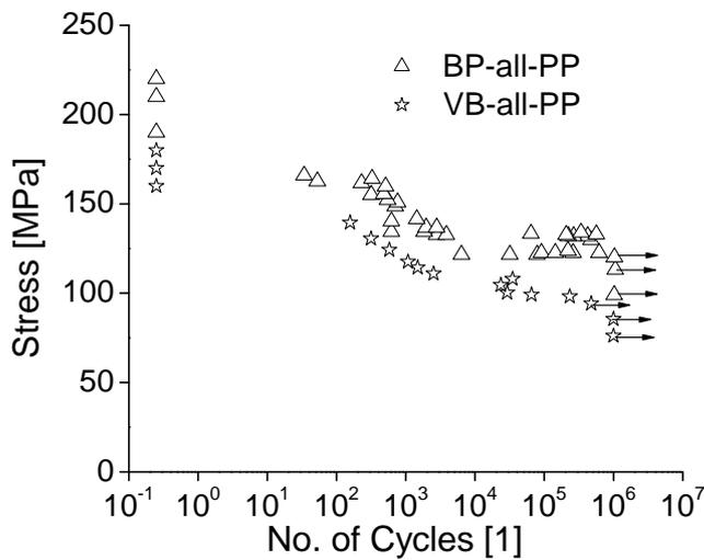
Figure 2. S-N curves for BP-all-PP, and VB-all-PP woven composites, tested at RT, illustrating the effect of consolidation pressure on the fatigue response. Arrows signify specimens that did not fail after  $10^6$  cycles.
