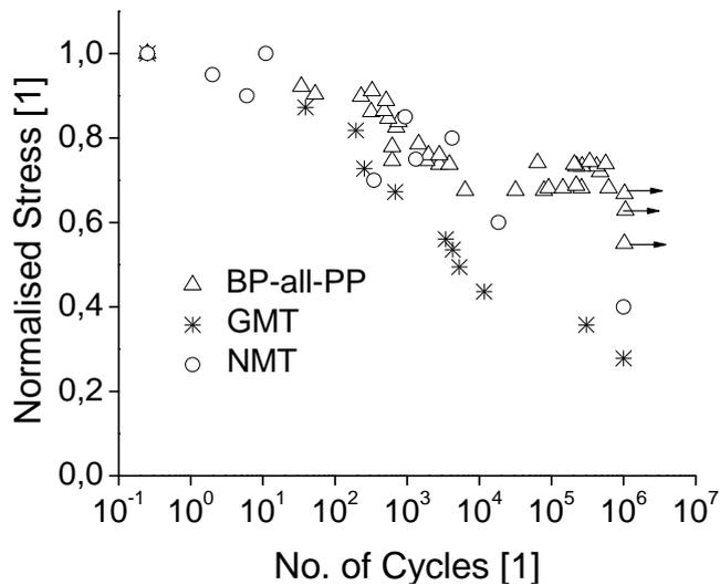
Figure 4. Normalised stress ( $\sigma/\sigma_0$ ) as a function of the number of cycles to failure, comparing the fatigue response and the damage development of BP-all-PP woven composites with GMT and NMT.  $\sigma_0$  corresponds to the UTS of respective material. Arrows signify specimens that did not fail after  $10^6$  cycles
