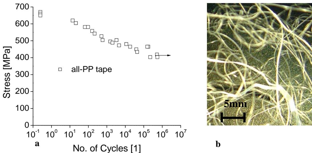
Figure 1. (a) Fatigue response of PP tapes at RT represented by S-N curves (arrows signify specimens that did not fail after  $10^6$  cycles) and (b) macroscopic image of a failed PP tape after failure, showing the completely fibrillated tape structure and no recognisable tape geometry remaining.
