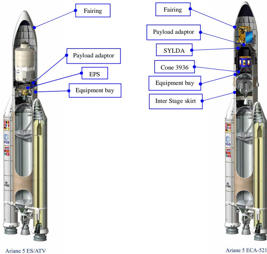
Figure 1: Composite structures on Ariane 5.
