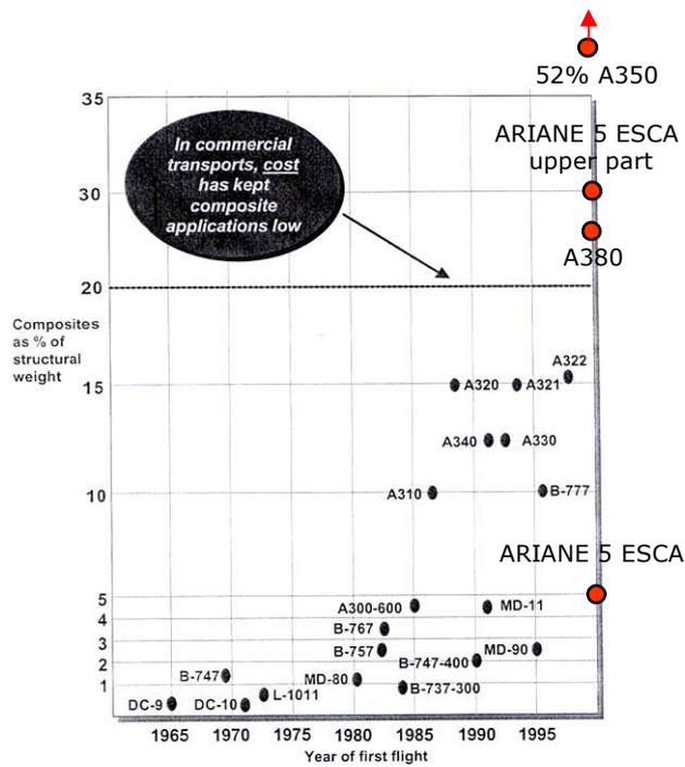
Figure 2: Ratio of composites for the main planes compared to the Ariane 5-ECA configuration.
