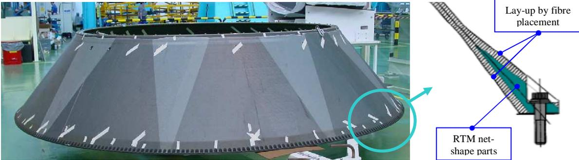
Figure 5: Cone 3936 and scheme for the cobonded integrated CFRP interface for the cone 3936.
