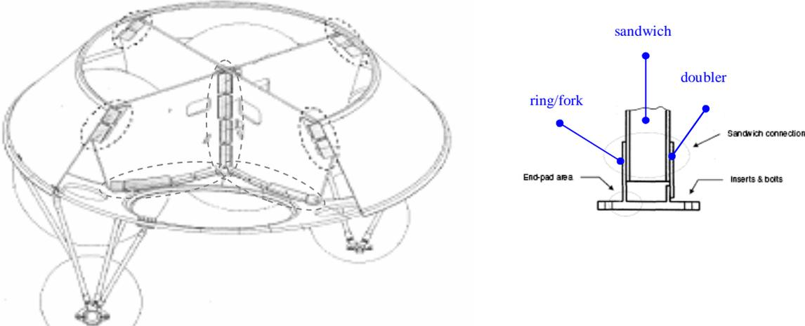
Figure 4: EPS configuration with Pi-fitting localisation (surrounded by dotted lines) and scheme of the connection.
