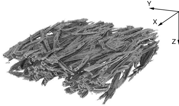
Figure 1: Surface rendering of fibres in a pulp-fibre composite material imaged in 3D using X-ray microtomography. The average cross-sectional diameter of the fibres is approximately 30 \mu\text{m} .
