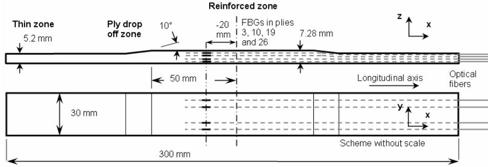
Figure 1. Plan of the technological specimen. Dimensions and FBG instrumentation.
