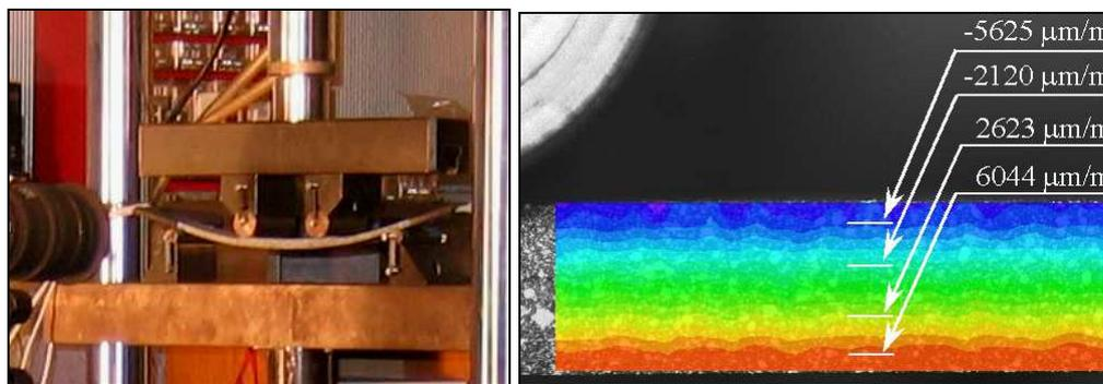
Figure 5. a) Multi-instrumented technological specimen submitted to a 4-point bending test. b) 3D DIC longitudinal strain field in the reinforcement zone for a 16 mm displacement
