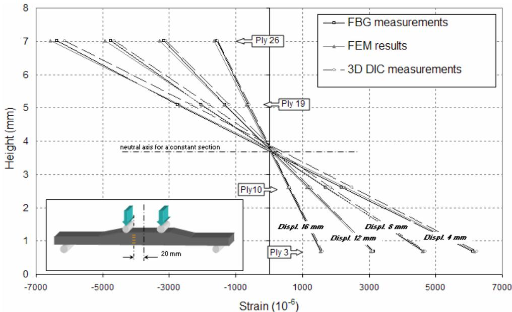
Figure 7. Through-the-thickness strain distribution for displacements of 4, 8, 12 and 16 mm. Comparison between FBGs, 3D-DIC, and FEM.
