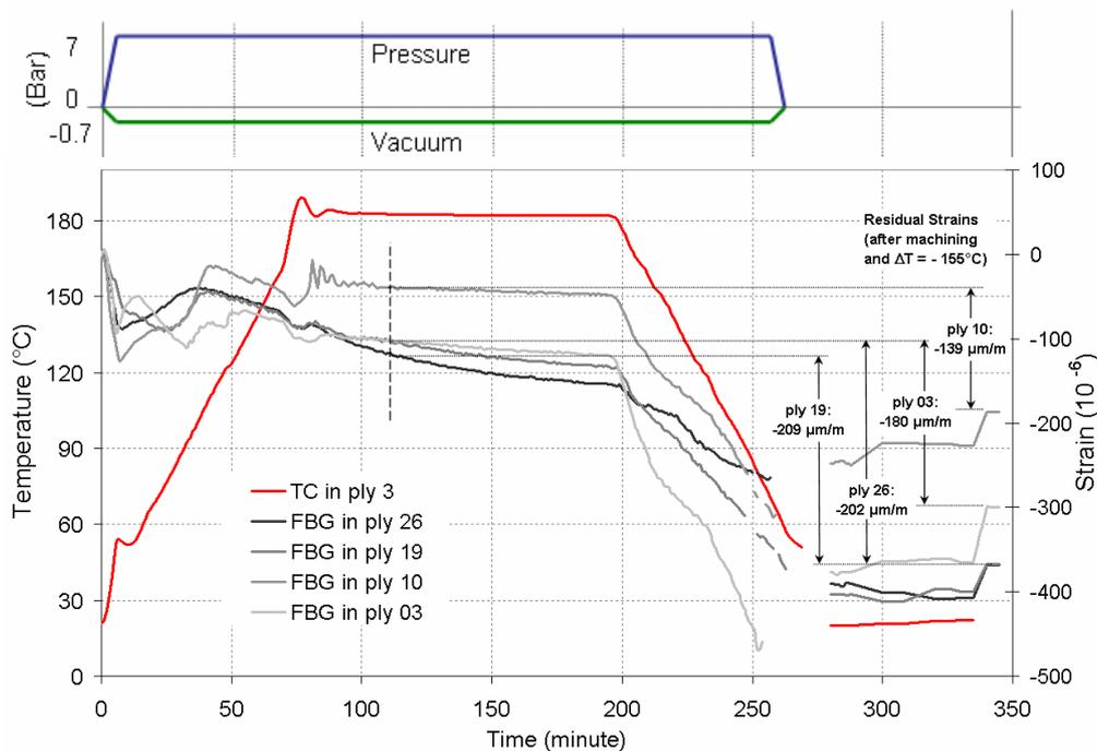
Figure 3. Process induced strain changes measured by FBGs through-the-thickness of the reinforced zone of the technological specimen during the autoclave cure cycle.
