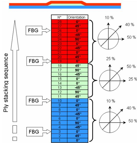
Figure 2. Ply stacking sequence of the technological specimen and position of embedded FBGs.
