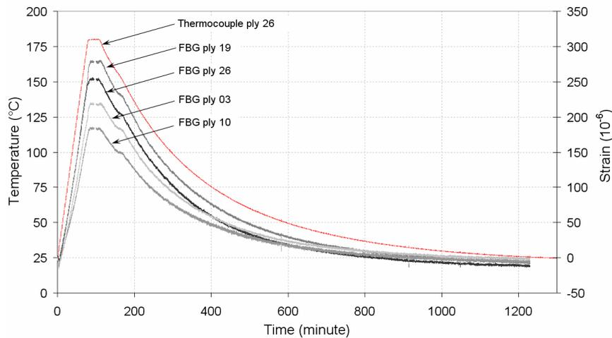
Figure 4. Thermally induced strain changes measured by FBGs through-the-thickness of the reinforced zone of the technological specimen during the oven reheating cycle.
