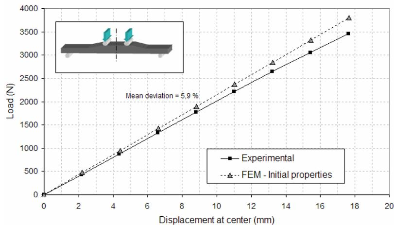
Figure 6. Load changes versus displacement for the 4-point bending test. Test – calculation comparison
